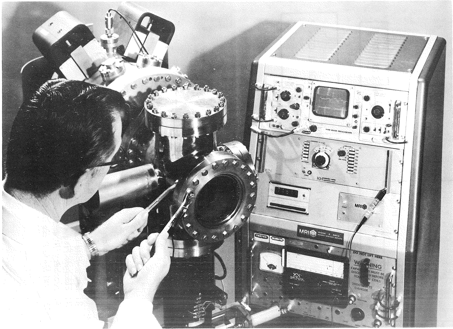
Figure 20 - Photograph of Prototype Instrumentation Being Used to Set Bolt Preloads on a Vacuum System.
