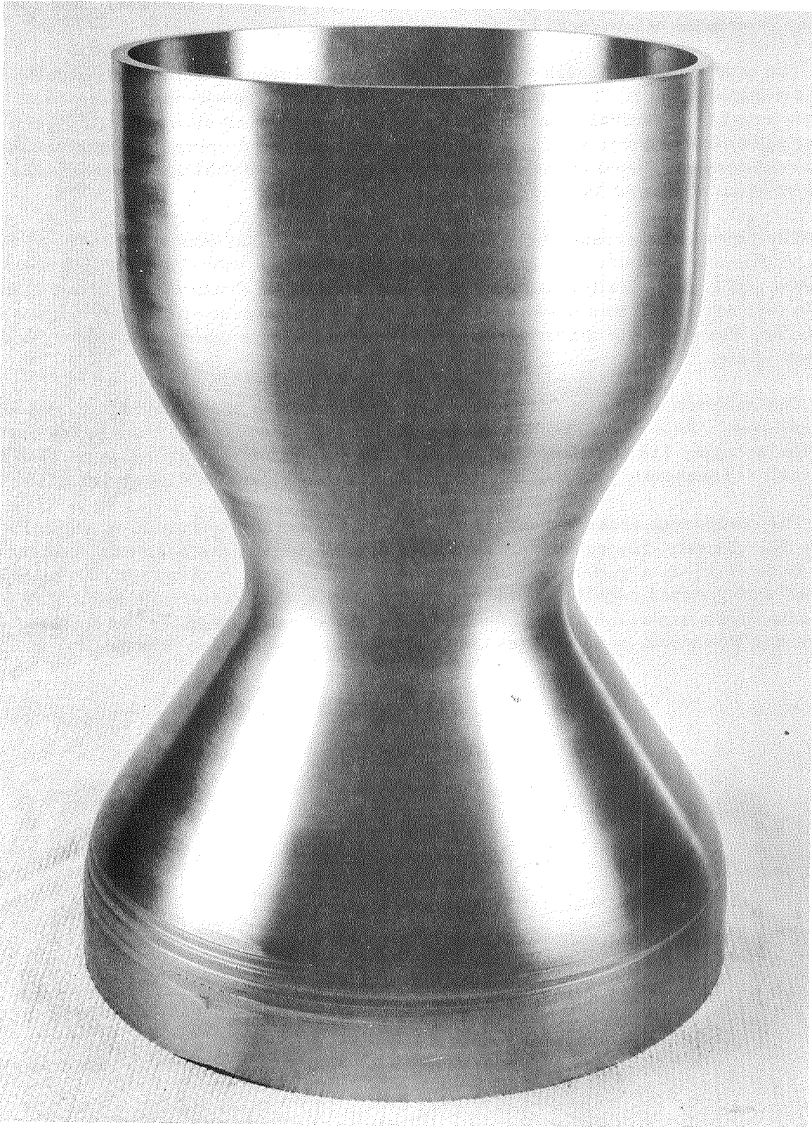
FIGURE 35. EXPLOSIVELY FORMED AND FINAL-MACHINED 304 SS NOZZLE SHELL
