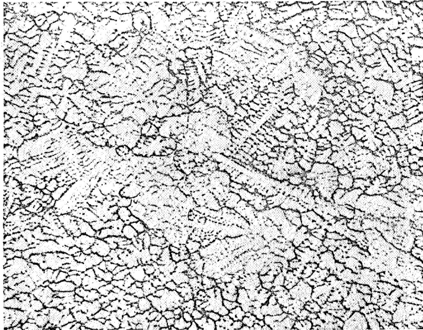
Figure IB5a - Macrostructure of remelted AS-30 No. 2. Tungsten completely alloyed in remelt as verified by improved metallographic technique. 25X
