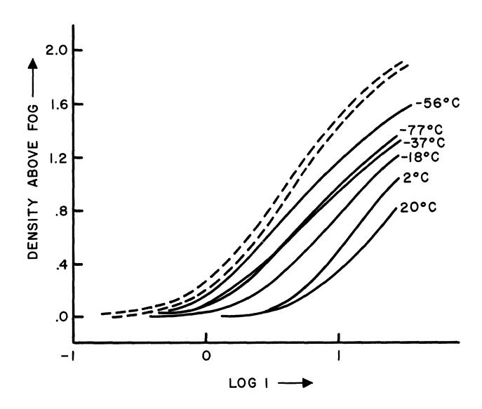
FIGURE 1 -- Characteristicscurves for Tri-X (solid lines) and 103a-0 (dashed lines) at various temperatures for  $\lambda$ =4400A and t=30 min.
