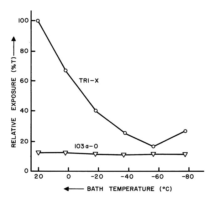
FIGURE 2 -- Relative exposure (in % transmission normalized to Tri-X at 20°C) needed to produce a density of 0.6 above fog as a function of bath temperature.
