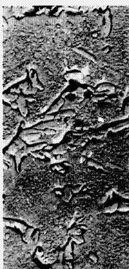
Figure 16. Electron Micrographs of Inconel 718 in the 1725 F, 1500 - 1200 F Heat Treatment Condition. Etchants: 92 HCl, 3 HNO 3 , 1/2 H 2 SO 4 (3000x)
