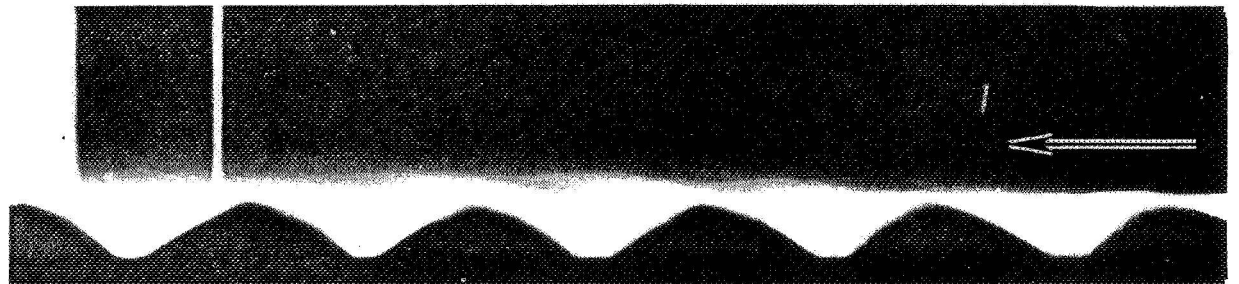
FIGURE 26 53 TO 63 MICRON DIA \text{SiO}_2 ROUGH SURFACE AT THRESHOLD CONDITIONS. q_\infty = 1.34 \times 10^{-3} \text{LB/IN.}^2
