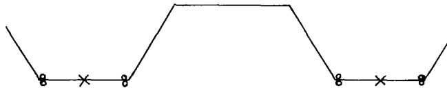
(d) Idealization of (c) used in the analysis: Point attachments at the ends of the trough lines, and point attachments permitting longitudinal sliding at the junctions of the trough plate elements and the inclined plate elements.
