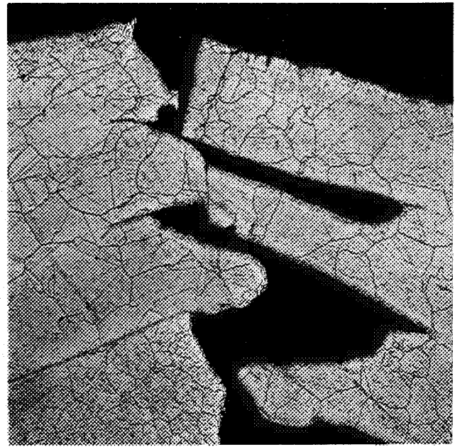
Figure 71. Photomicrographs of longitudinal failure sections in test vane No. 2 (magn: 100X).
