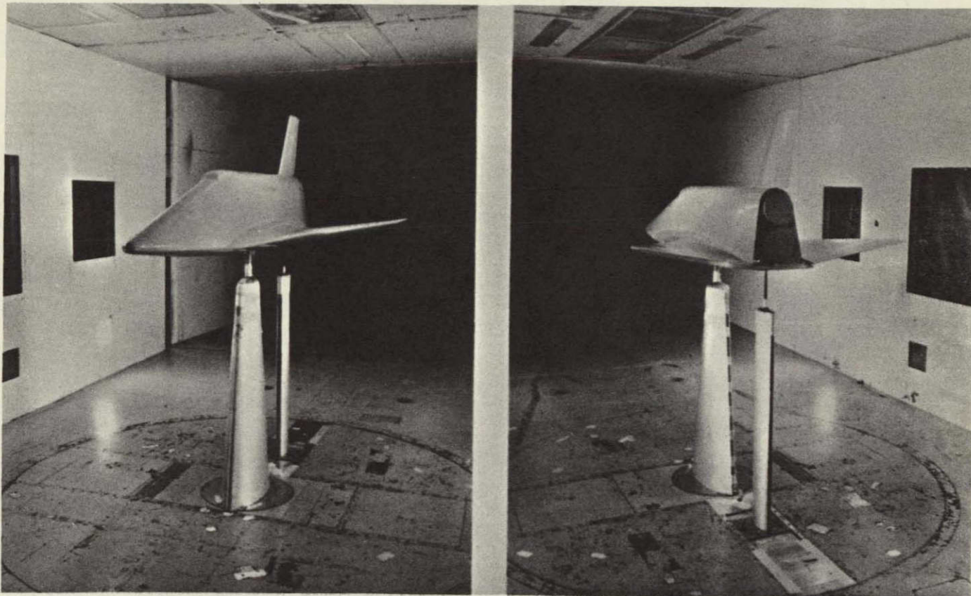
MCAIR LSWT Test 248 - Front and rear view of the model installed in the MCAIR Low Speed Wind Tunnel. Config. B 5 W 11 V 6 \delta e = -5^\circ , \delta a = 0^\circ \delta R = 0^\circ \delta SB = 0^\circ \delta BF = 0^\circ
