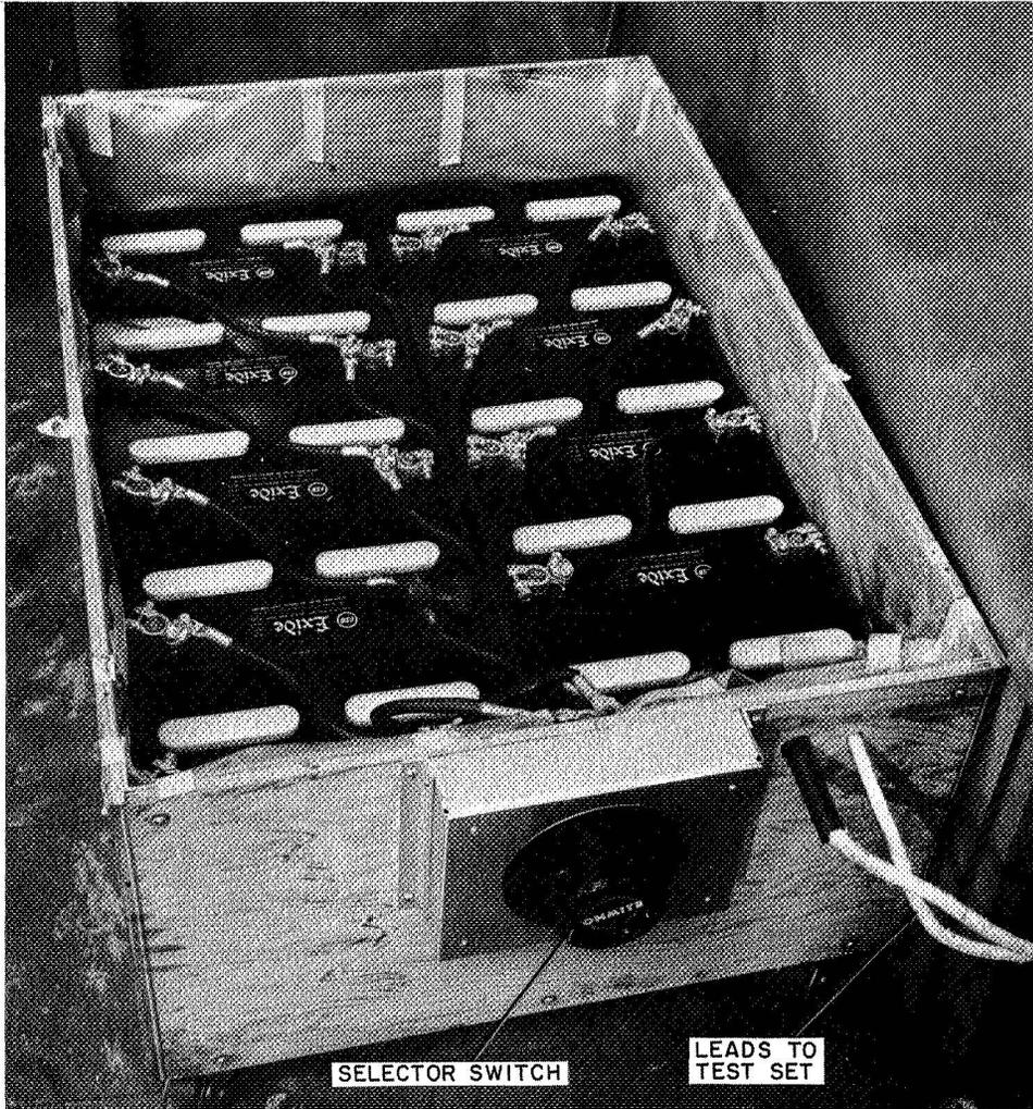
Figure 18 - Battery DC Voltage Supply
