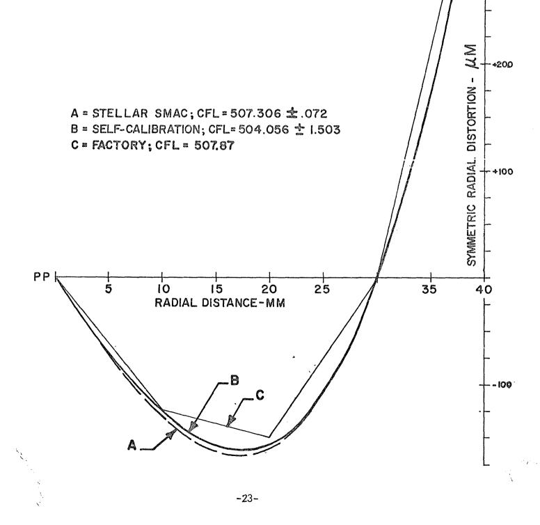
the region between 5 and 20mm radial distance where the difference between the curves is 5 to  $6 \mu m$ . However, a very slight rebalancing would have the two curves lie completely within their respective one sigma error bounds.
