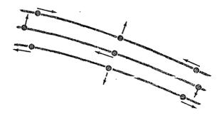
FIGURE 3. Simulated Photographic Sequence For Pure Self-calibration. Orbits are consecutive and of low inclination; spacecraft pitch maneuver allows 80° angle of convergence between end photographs. Arrows indicate camera is rotated 90° between individual exposures.
