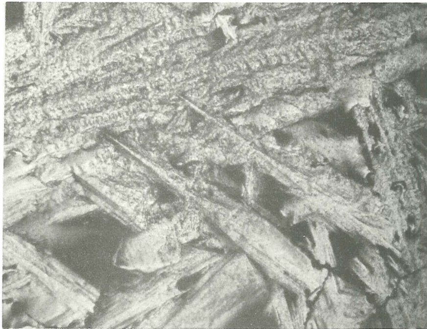
(a) S-11(b), InSb Film Annealed at 540°C for 3 min, 3.5 \mu\text{m} Thick, 50 Magnification
