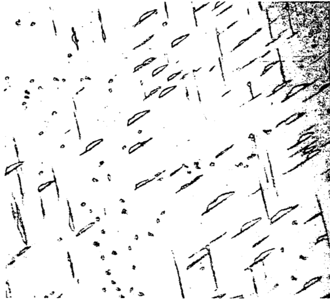
Figure 25. ACICULAR STRUCTURE ON 362 EMITTER SURFACE AFTER ETCHING
