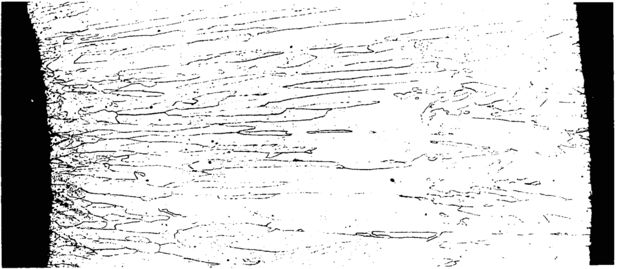
Figure 36. MICROSTRUCTURE OF AS-DEPOSITED C1-CVD-W, SAMPLE No. 8 (EMITTER 363)
