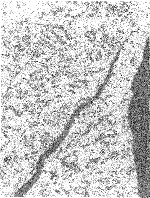
Microstructure of the Failed Ball at the Ball Outer Edge
