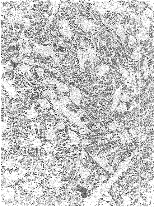
Microstructure of a Ball Adjacent to the Failed Ball Center
