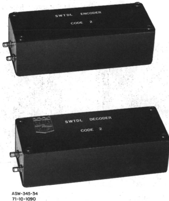
Figure 4-6. Code 2 Surface Wave Devices (Encoder and Decoder)
