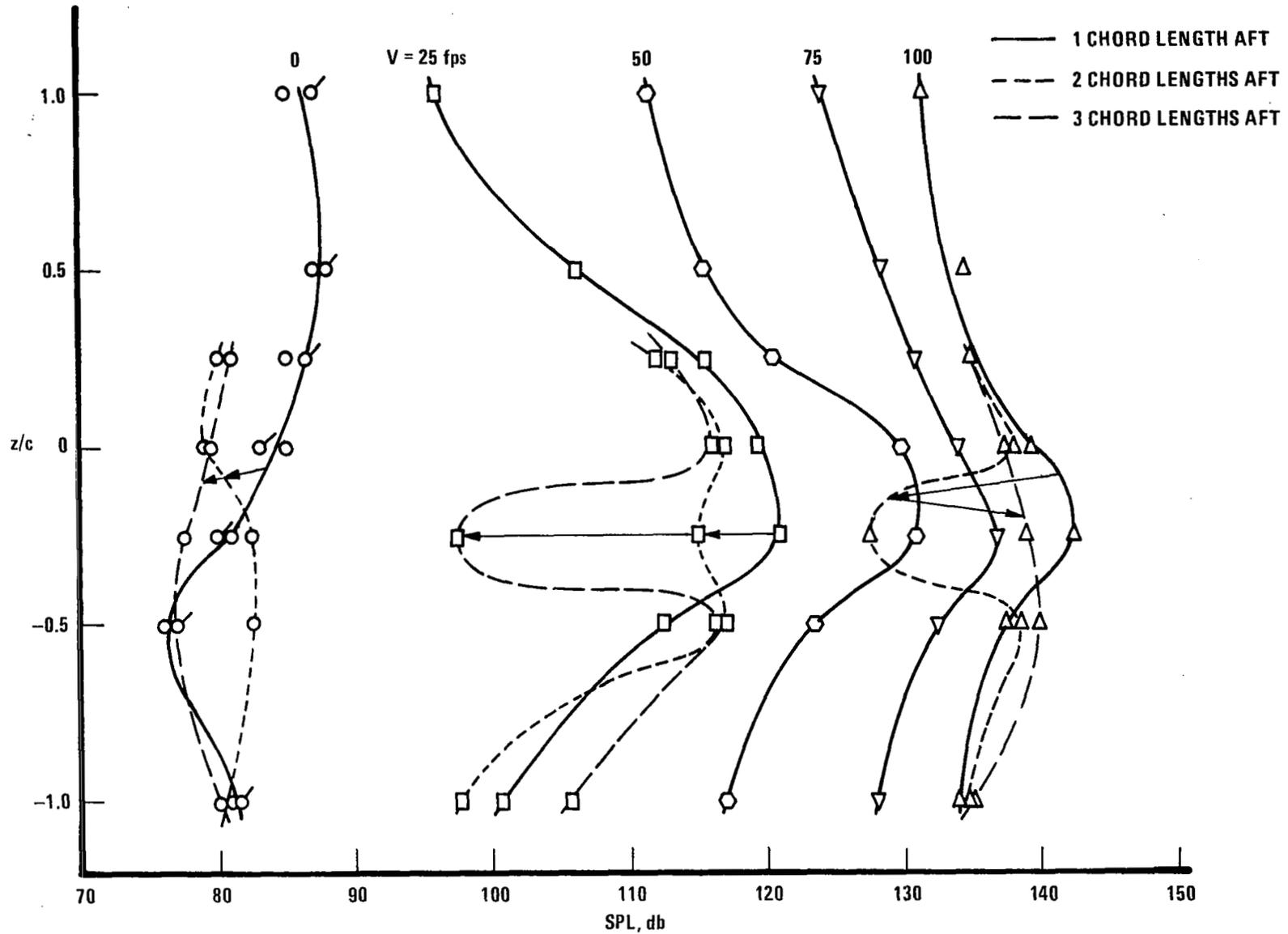
Figure 7. Variation of peak sound pressure level at the fundamental frequency in the vertical centerline plane at three positions aft of the trailing edge of an oscillating, two-dimensional NACA 0012 airfoil.  $f = 16$  Hz.;  $\alpha = 12^\circ$ ;  $\Delta\alpha = \pm 3^\circ$ .
