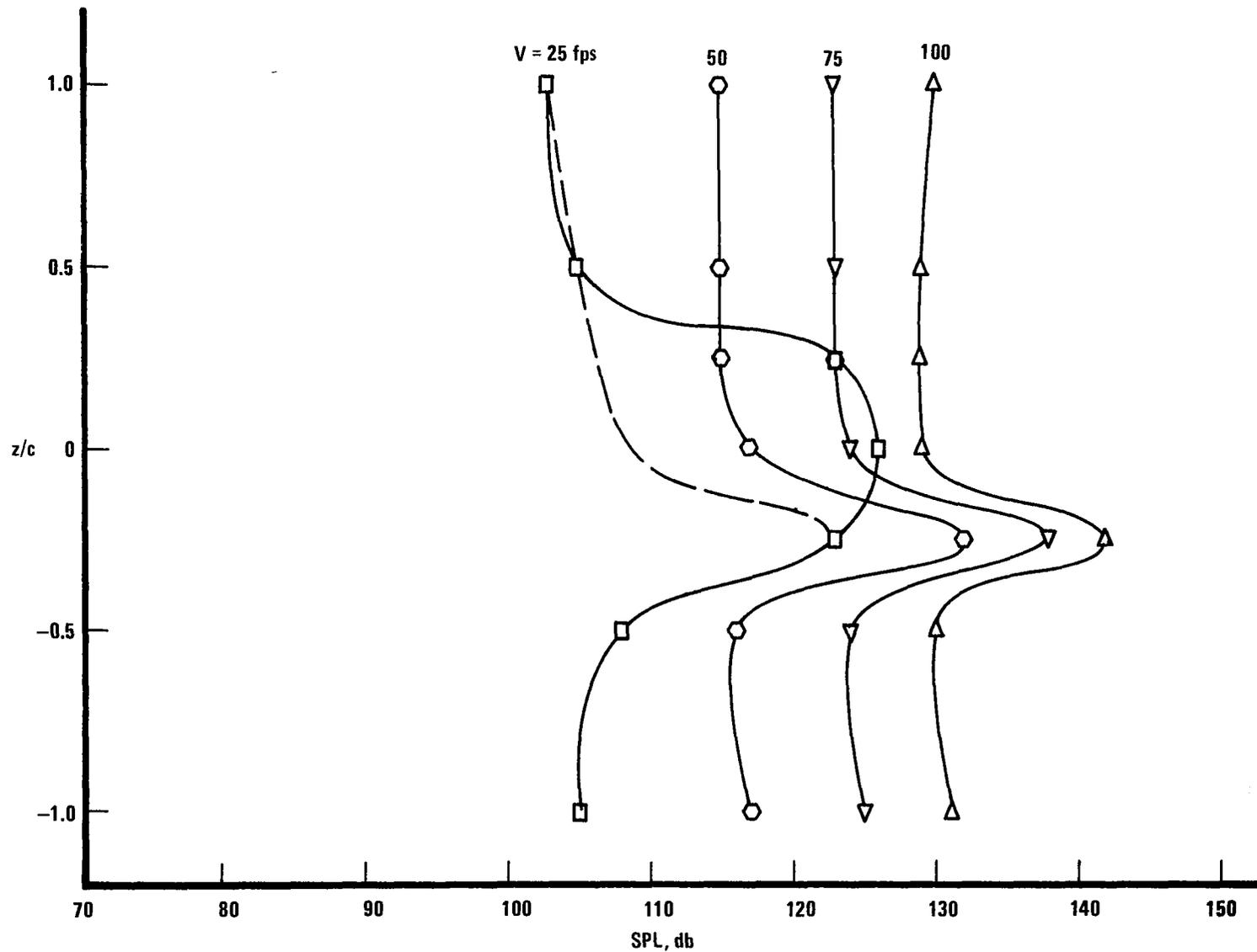
Figure 17. Variation of overall sound pressure level in the vertical centerline plane at one chord length aft of the trailing edge of a two-dimensional NACA 0012 airfoil.  $f = 0$  Hz.;  $\alpha = 12^\circ$ .
