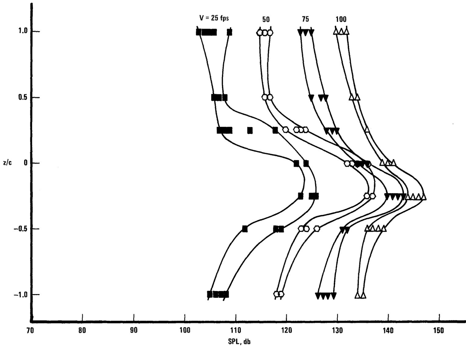
Figure 18. Variation of overall sound pressure level in the vertical centerline plane at one chord length aft of the trailing edge of an oscillating, two-dimensional NACA 0012 airfoil.  $f = 16, 20, 24, 28, 32$  Hz.;  $\alpha = 12^\circ$ ;  $\Delta\alpha = \pm 3^\circ$ .
