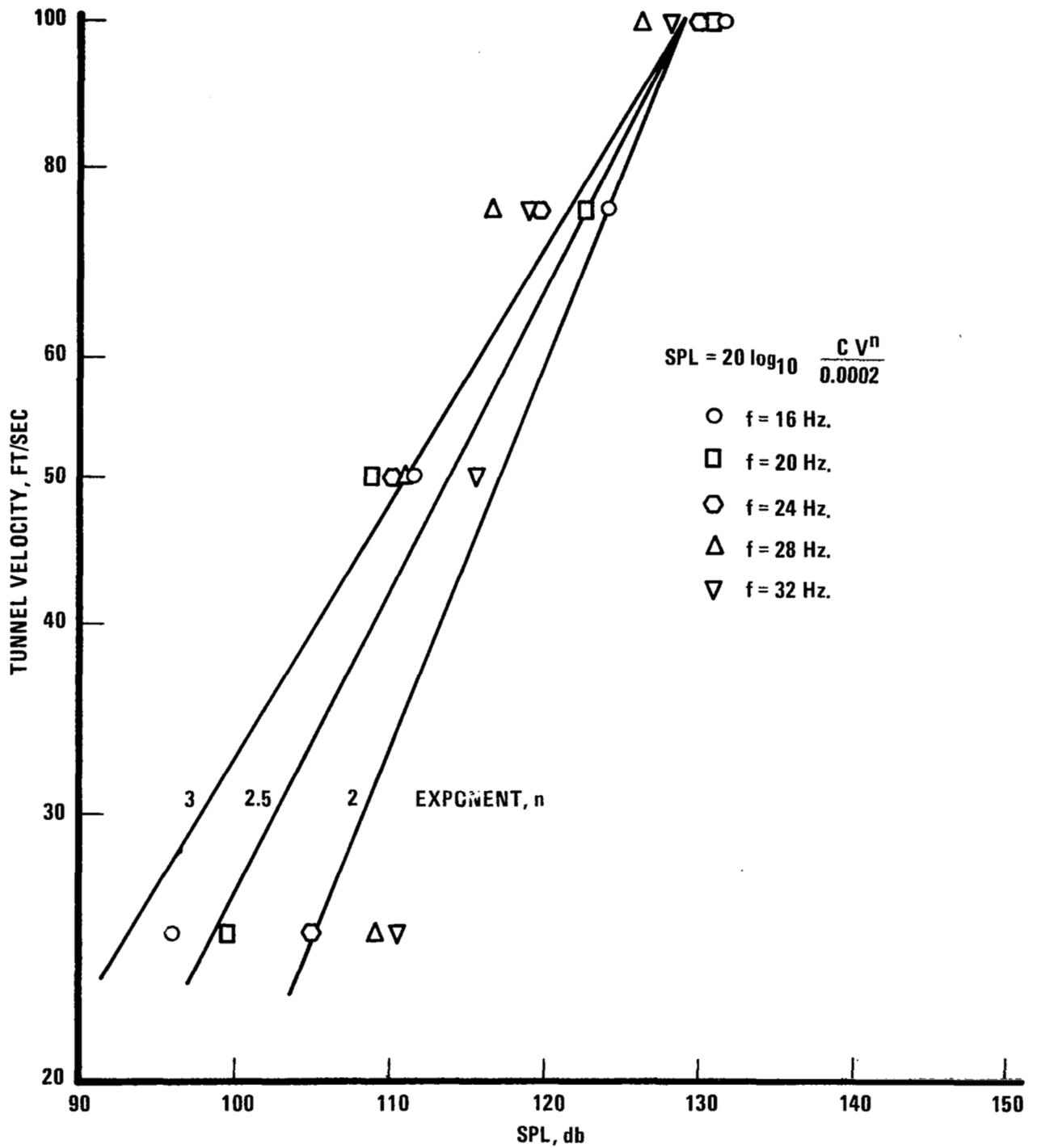
Figure 21. Peak sound pressure level at the fundamental frequency as a function of velocity behind the trailing edge of an oscillating, two-dimensional NACA 0012 airfoil.  $z/c = 1.0$ ;  $x/c = 1.0$ ;  $\alpha = 12^\circ$ ;  $\Delta\alpha = \pm 3^\circ$ .
