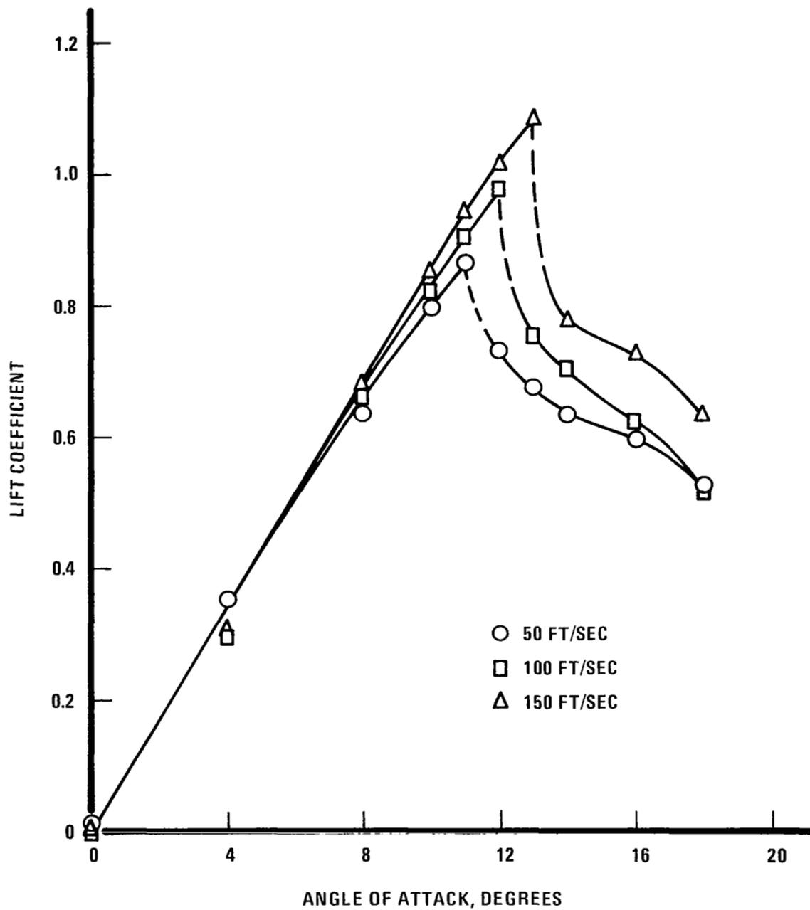
Figure 4. NACA 0012 Airfoil Lift Coefficient
