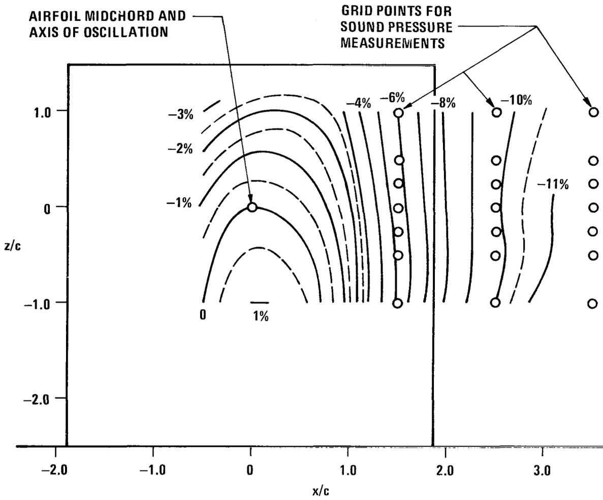
Figure 3. Lines of Constant Velocity Difference from Velocity at Airfoil Midchord Position in Longitudinal Center-line Plane with Airfoil Removed.  $V = 150$  Ft/Sec (Typical)
