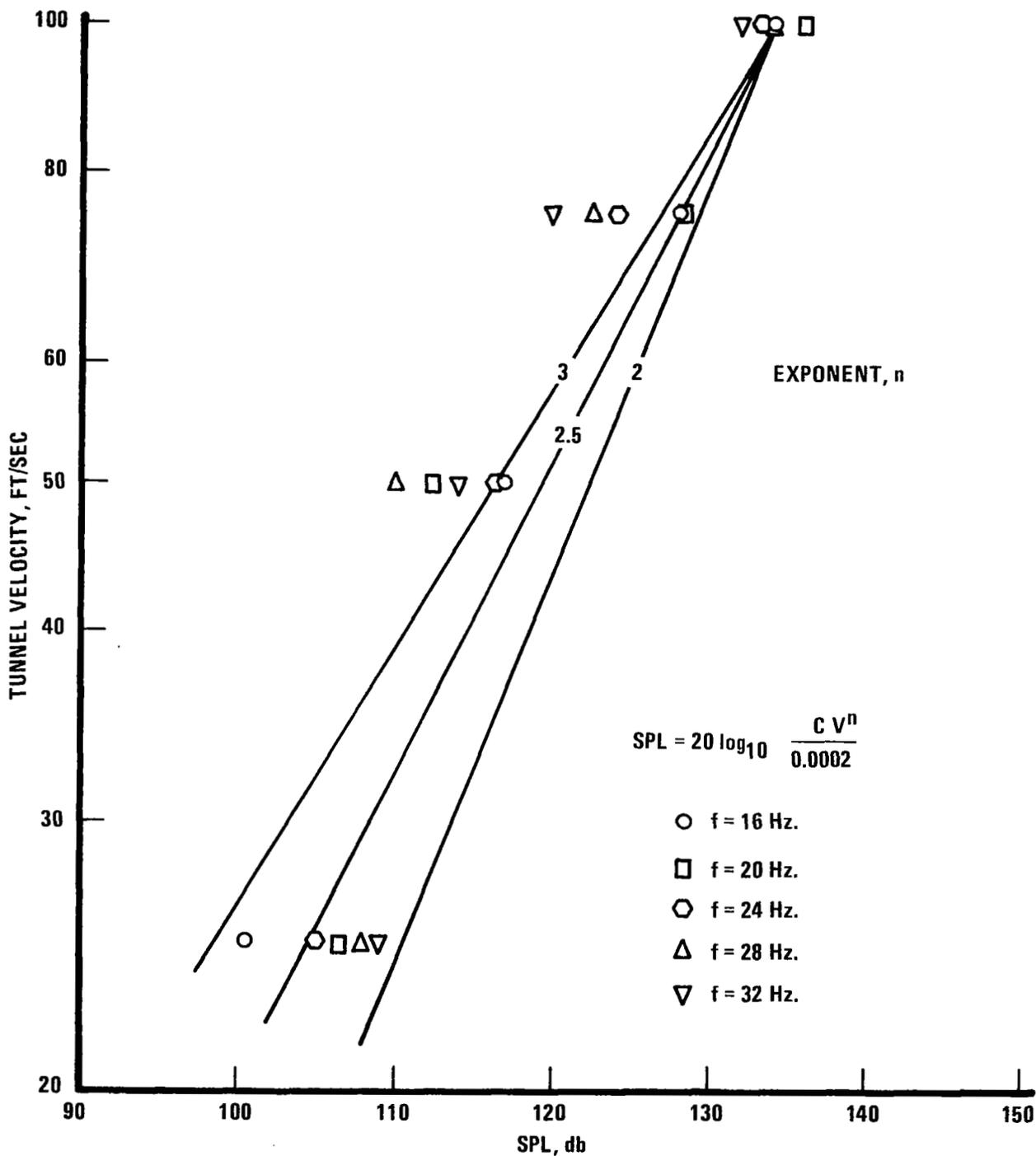
Figure 22. Peak sound pressure level at the fundamental frequency as a function of velocity behind the trailing edge of an oscillating, two-dimensional NACA 0012 airfoil.  $z/c = -1.0$ ;  $x/c = 1.0$ ;  $\alpha = 12^\circ$ ;  $\Delta\alpha = \pm 3^\circ$ .
