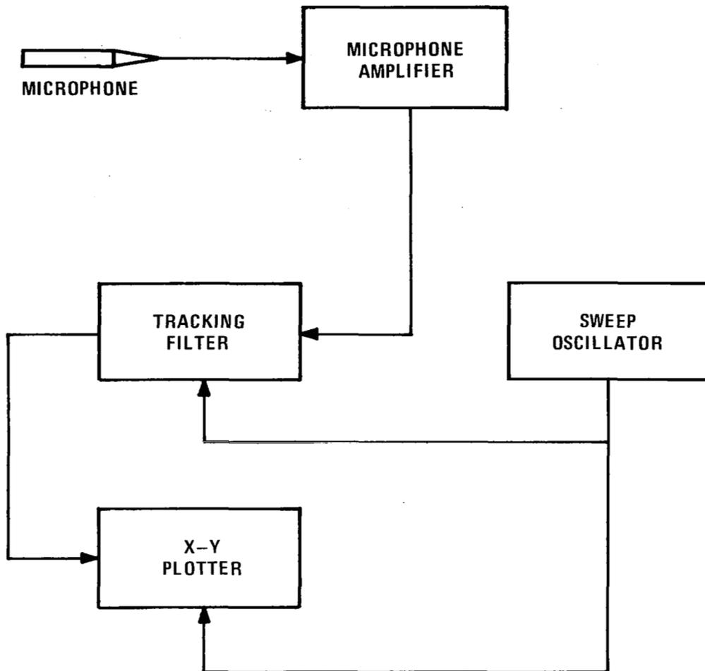
Figure 2. Flow Chart of Acoustic Measurement and Data Reduction.
