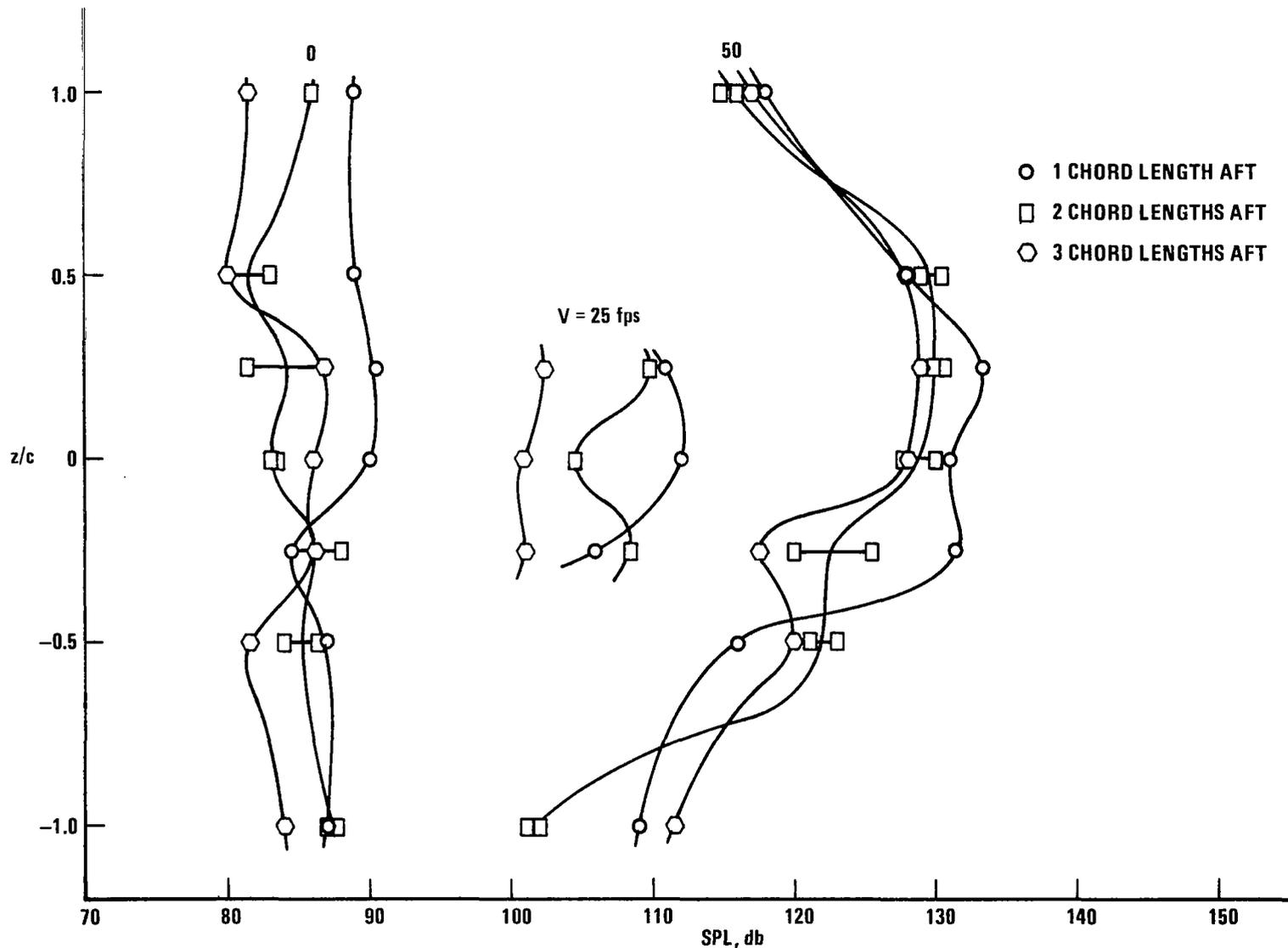
Figure 26. Variation of peak sound pressure level at the fundamental frequency in the vertical centerline plane at three positions aft of the trailing edge of an oscillating two-dimensional flat plate.  $f = 20$  Hz.;  $\alpha = 12^\circ$ ;  $\Delta\alpha = \pm 3^\circ$ .
