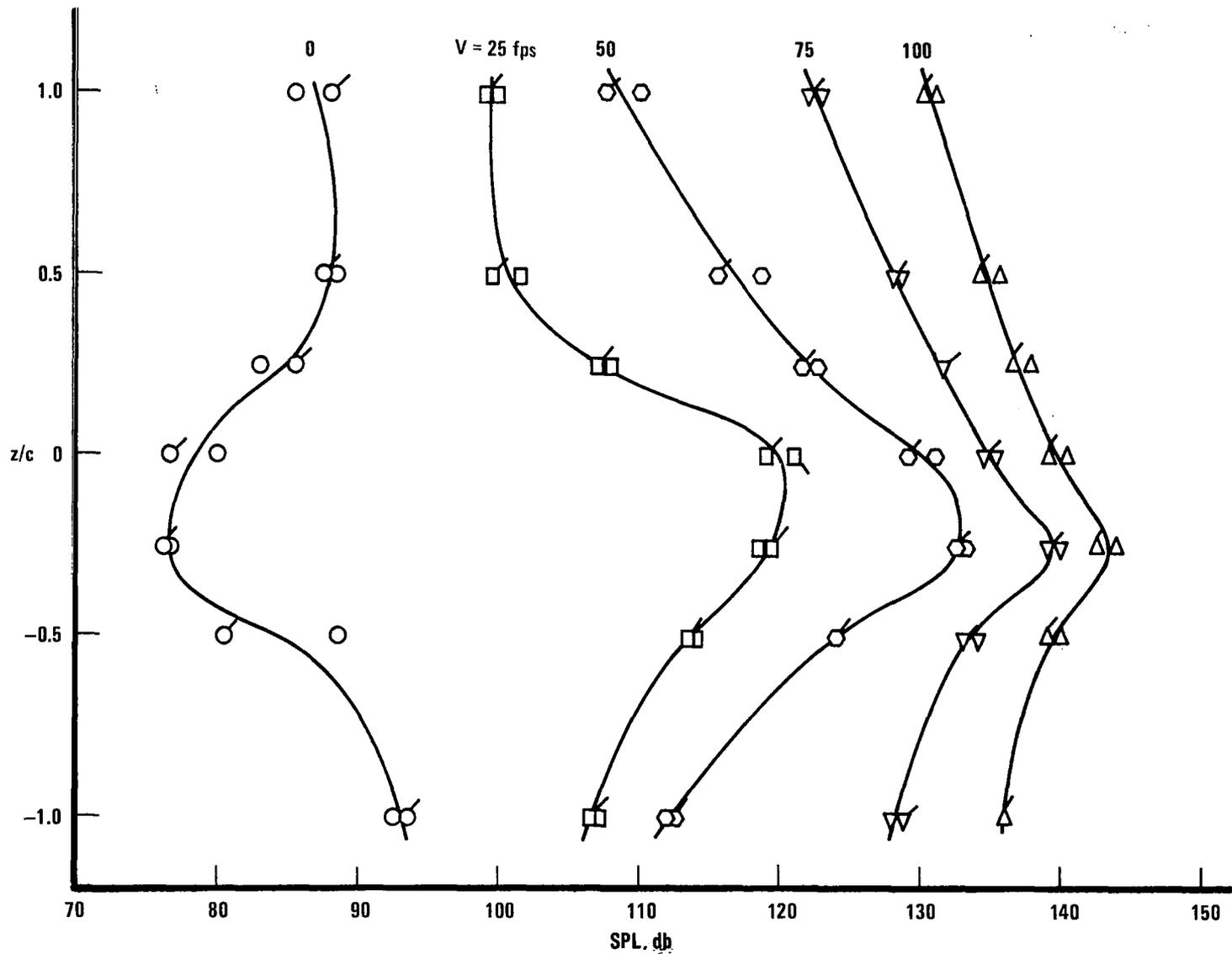
Figure 8. Variation of peak sound pressure level at the fundamental frequency in the vertical centerline plane at one chord length aft of the trailing edge of an oscillating, two-dimensional NACA 0012 airfoil.  $f = 20$  Hz.;  $\alpha = 12^\circ$ ;  $\Delta\alpha = \pm 3^\circ$ .
