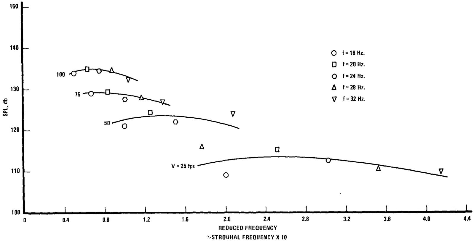
Figure 25. Peak sound pressure level at first harmonic of the fundamental frequency as a function of reduced frequency behind the trailing edge of an oscillating, two-dimensional NACA 0012 airfoil.  $x/c = 1.0$ ;  $\alpha = 12^\circ$ ;  $\Delta\alpha = \pm 3^\circ$ .
