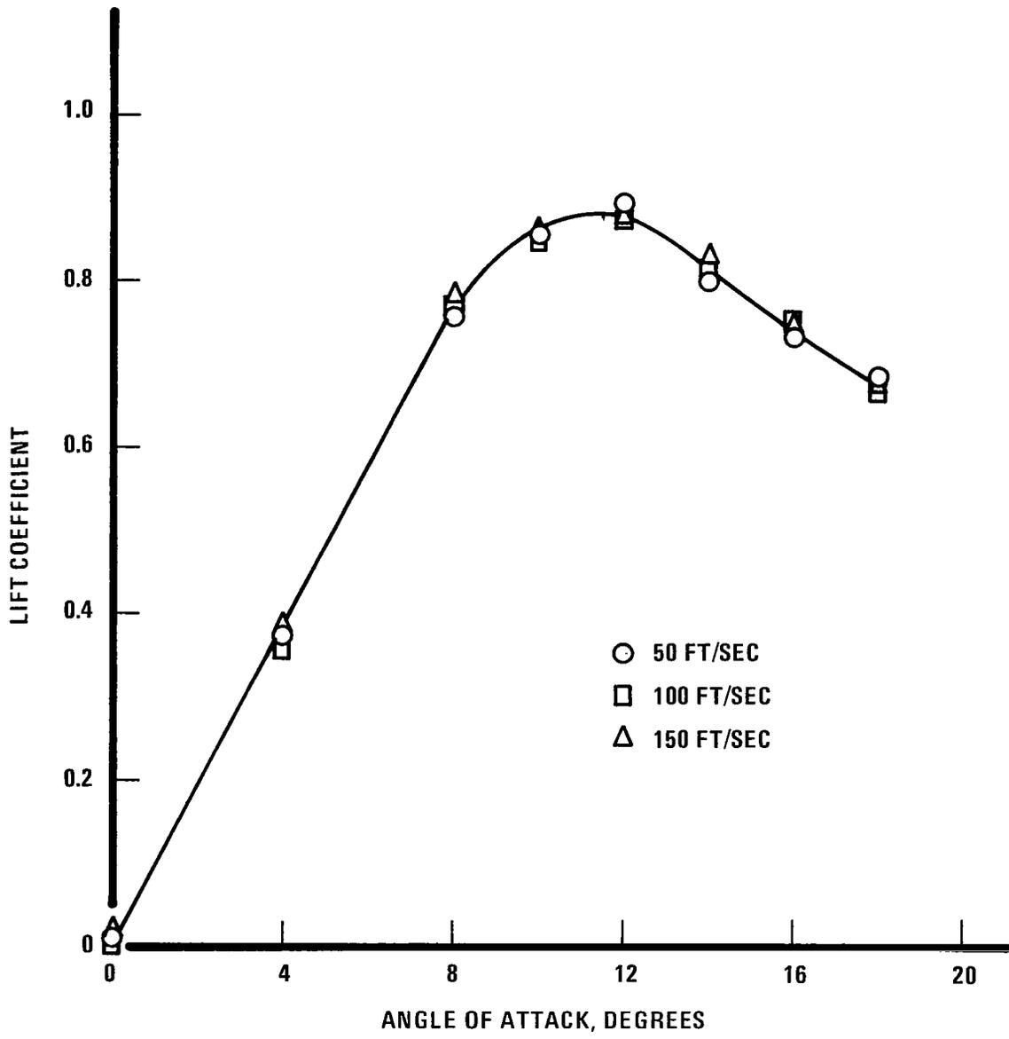
Figure 5. Flat Plate Lift Coefficient
