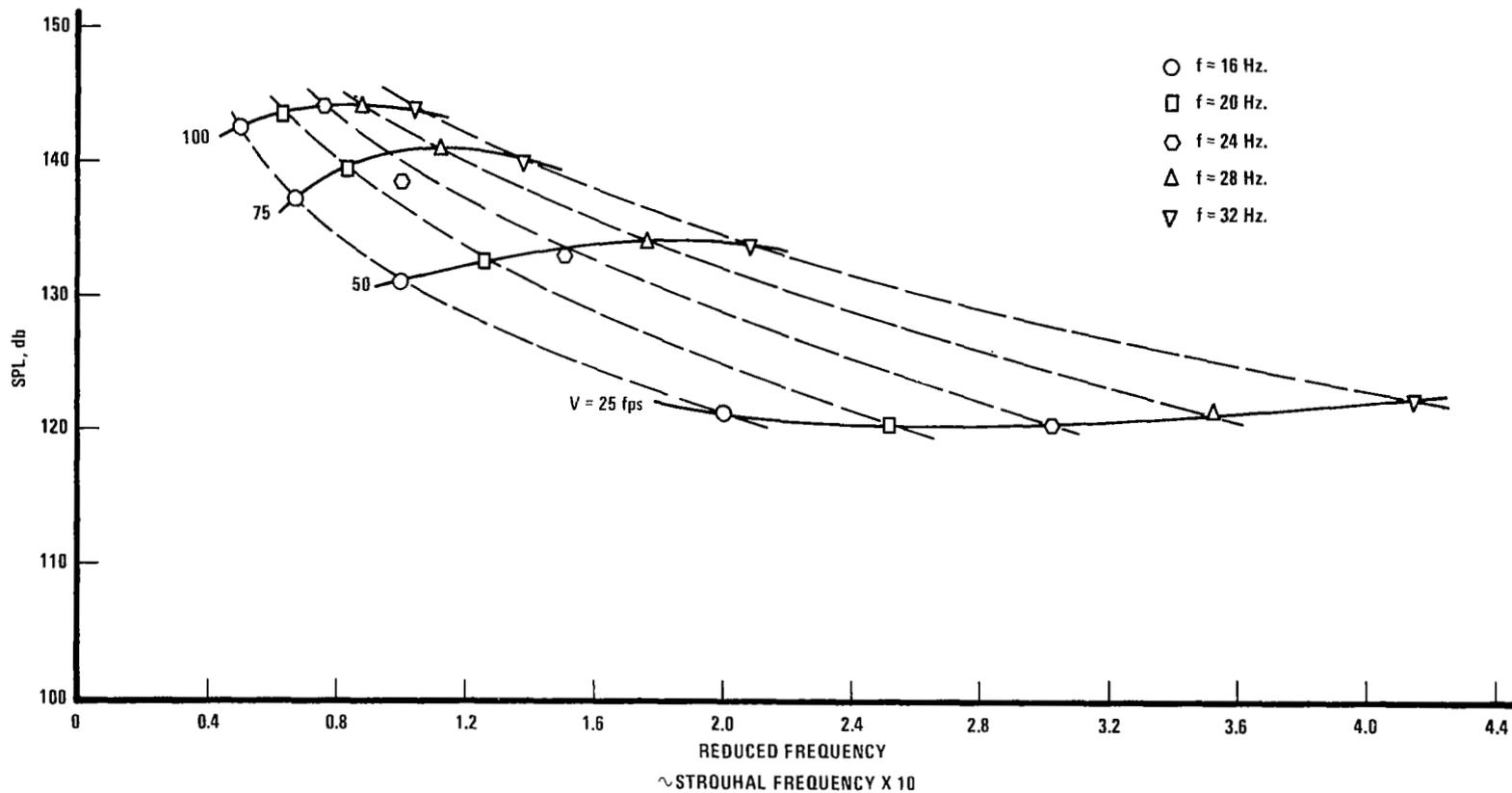
Figure 24. Peak sound pressure level at the fundamental frequency as a function of reduced frequency behind the trailing edge of an oscillating, two-dimensional NACA 0012 airfoil.  $x/c = 1.0$ ;  $\alpha = 12^\circ$ ;  $\Delta\alpha = \pm 3^\circ$ .
