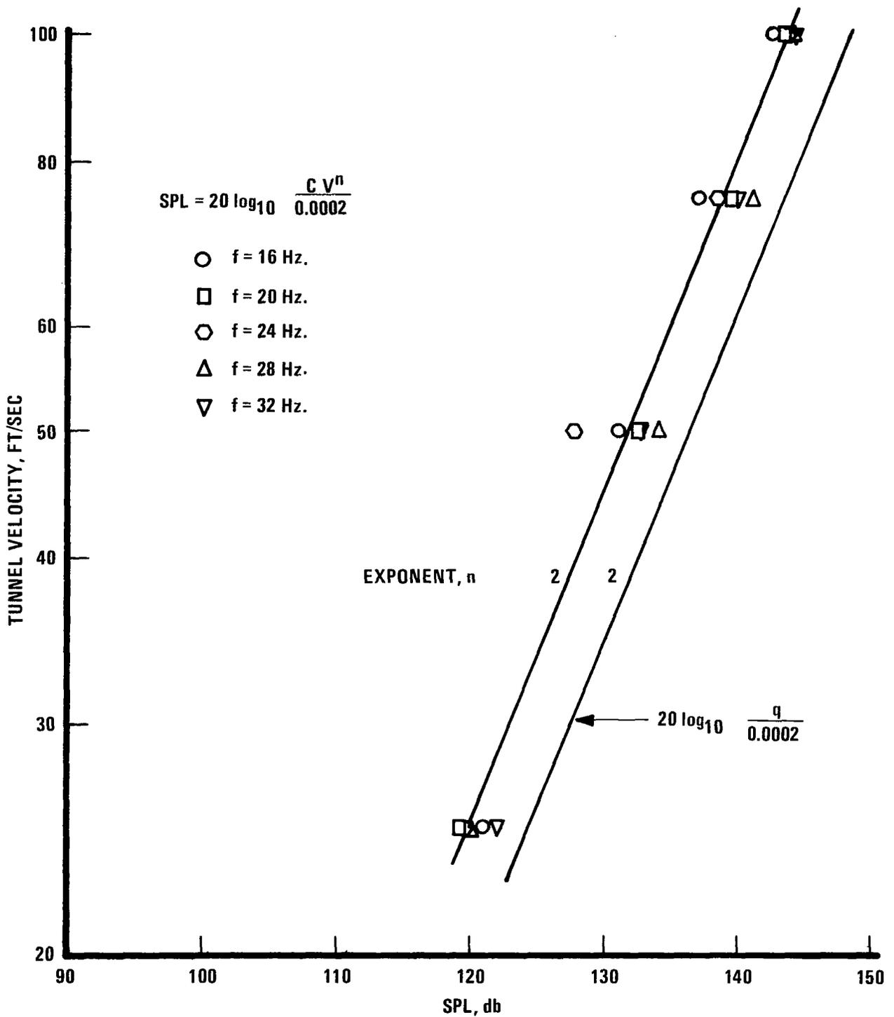
Figure 19. Peak sound pressure level at the fundamental frequency as a function of velocity behind the trailing edge of an oscillating, two-dimensional NACA airfoil.  $z/c = -0.25$ ;  $x/c = 1.0$ ;  $\alpha = 12^\circ$ ;  $\Delta\alpha = \pm 3^\circ$ .
