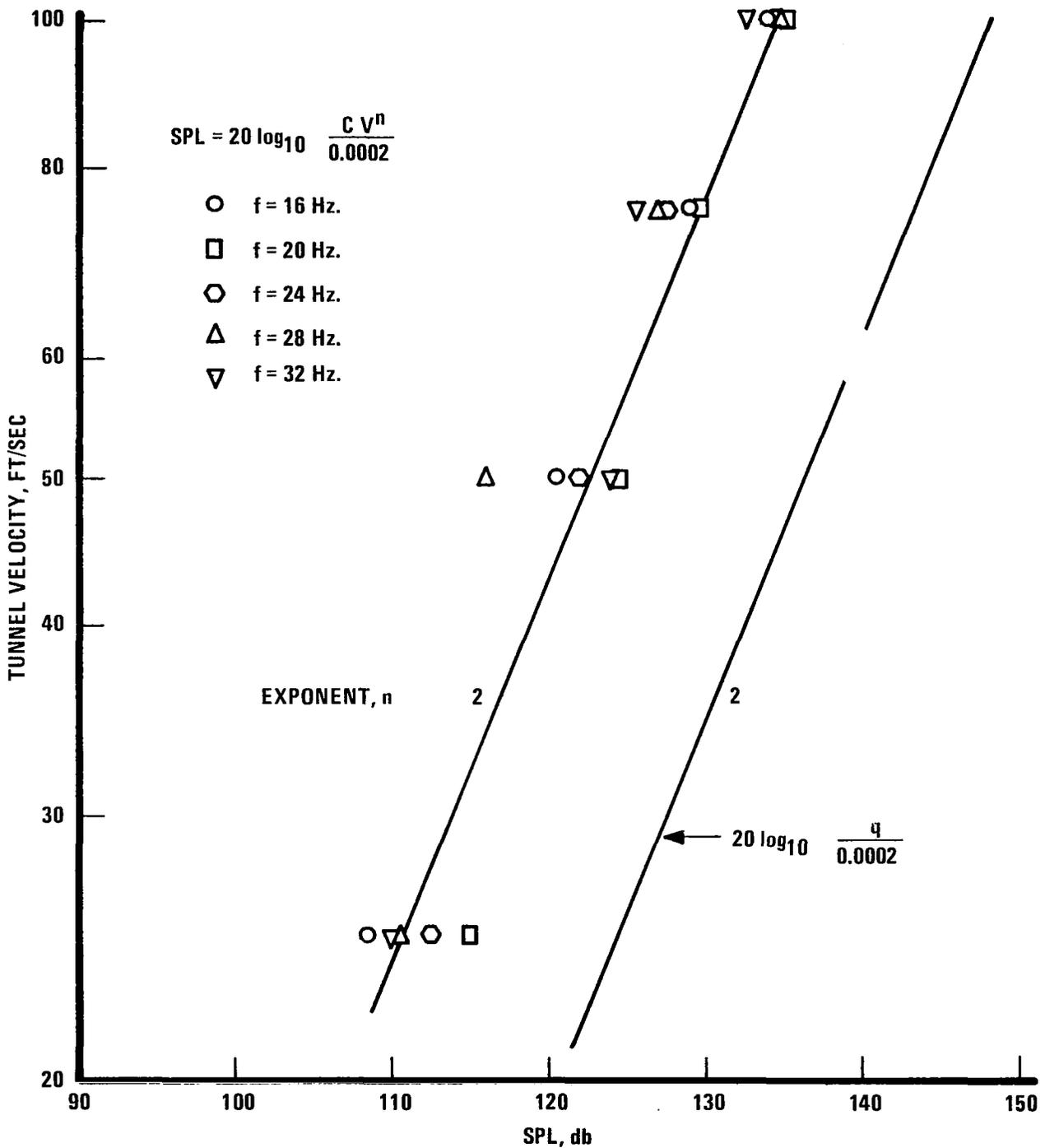
Figure 20. Peak sound pressure level at first harmonic of the fundamental frequency as a function of velocity behind the trailing edge of an oscillating, two-dimensional NACA airfoil.  $z/c = -0.25$ ;  $x/c = 1.0$ ;  $\alpha = 12^\circ$ ;  $\Delta\alpha = \pm 3^\circ$ .
