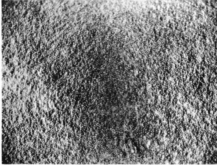
Figure 3-112 TUNGSTEN MICROSPHERES ON SURFACE OF FLIGHT SAMPLE 10 (10F-00) AFTER REMOVAL FROM CAPSULE
