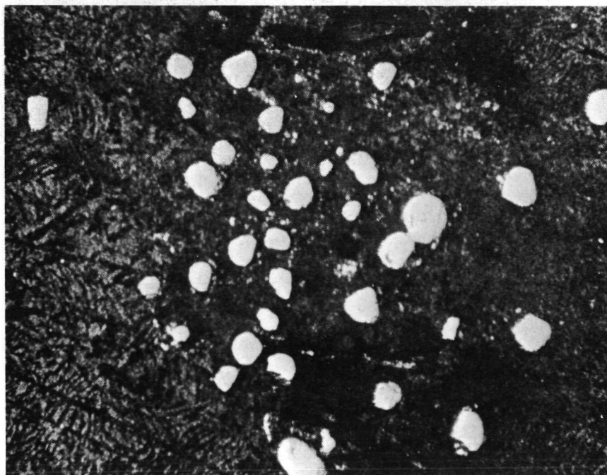
Figure 3-106 MASSIVE EUTECTIC STRUCTURE OBSERVED IN CONTROL SAMPLE 10 SECTION 10C-A-005
