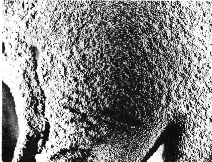
Figure 3-103 TUNGSTEN MICROSPHERES ON SURFACE OF CONTROL SAMPLE 10 (10C-00) AFTER REMOVAL FROM CAPSULE
