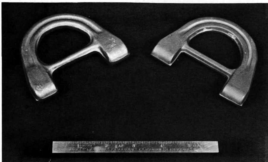
FIGURE 22.—Ti-6Al-4V powder forging preforms (pressed and sintered). Part is cargo tie-down ring for Lockheed C5A. (Courtesy Nuclear Materials and Equipment Corp.)
