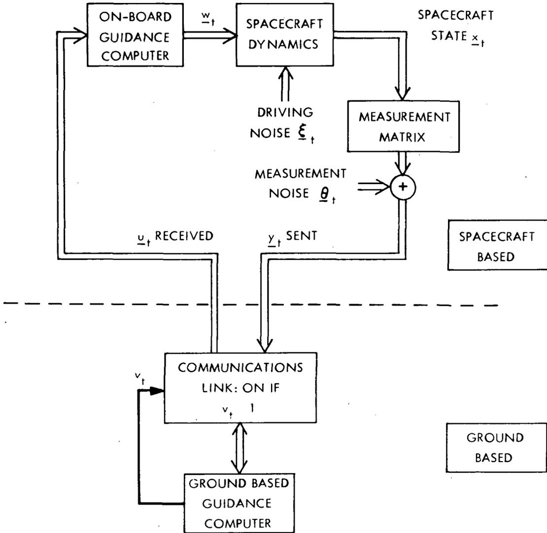
Fig. 6.1 System Structure
