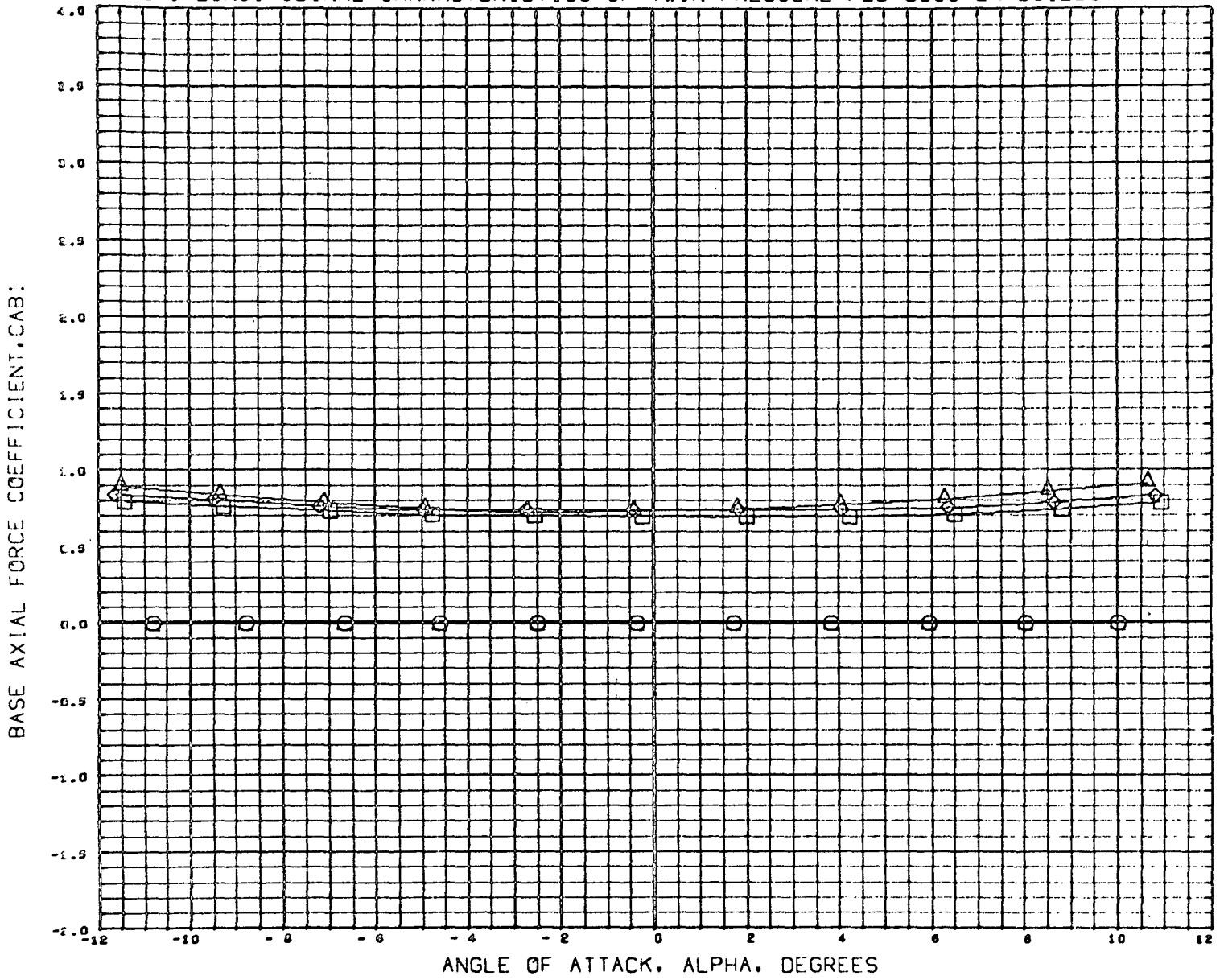
FIGURE-1 LONGITUDINAL CHARACTERISTICS OF TWIN PRESSURE FED BOOSTER BUILDUP
