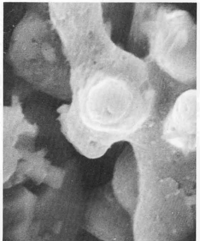
FIGURE 35. SEM PHOTOMICROGRAPHS OF CYCLED ELECTRODE MADE FROM ISOSTATICALLY COMPACTED PLAQUE, INCO 287 POWDER, 80 % 25 \mu
