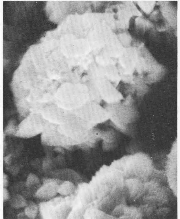
FIGURE 20. SEM PHOTOMICROGRAPHS OF CYCLED ELECTRODES MADE FROM ISOSTATICALLY COMPACTED PLAQUES, 60 % 25 \mu .
