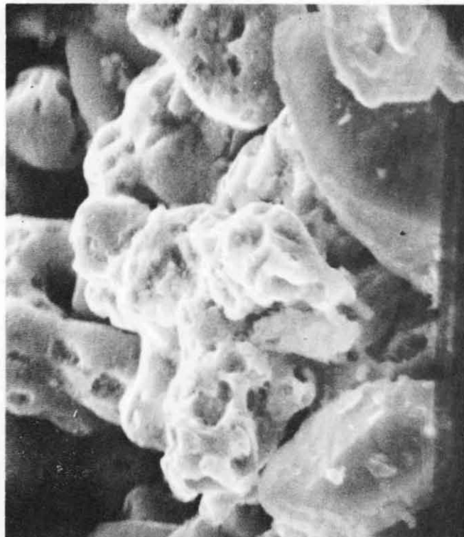
FIGURE 37. SEM PHOTOMICROGRAPHS OF CYCLED ELECTRODE MADE FROM ISOSTATICALLY COMPACTED PLAQUE, INCO 287 POWDER, 80 % 50 \mu
