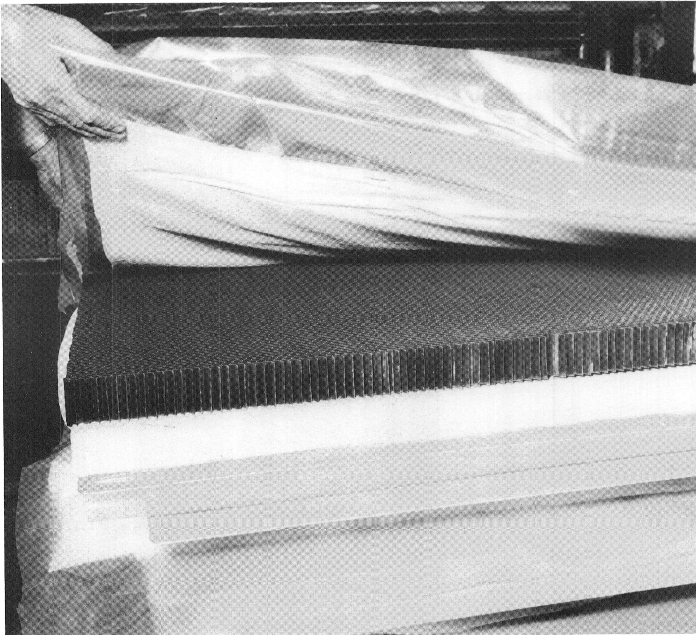
Figure 19. Closeup of -13 Subassembly After Bond Showing Porous Felt Paper and Teflon Cloth
