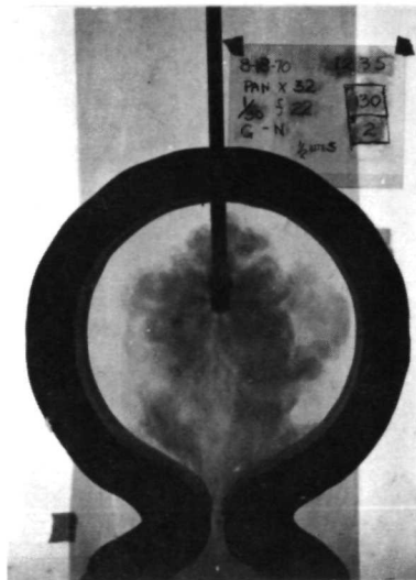
Fig. 5.4 High velocity injector results at varying injector nozzle position. All outer flows 130 cfm, inner 2 cfm
