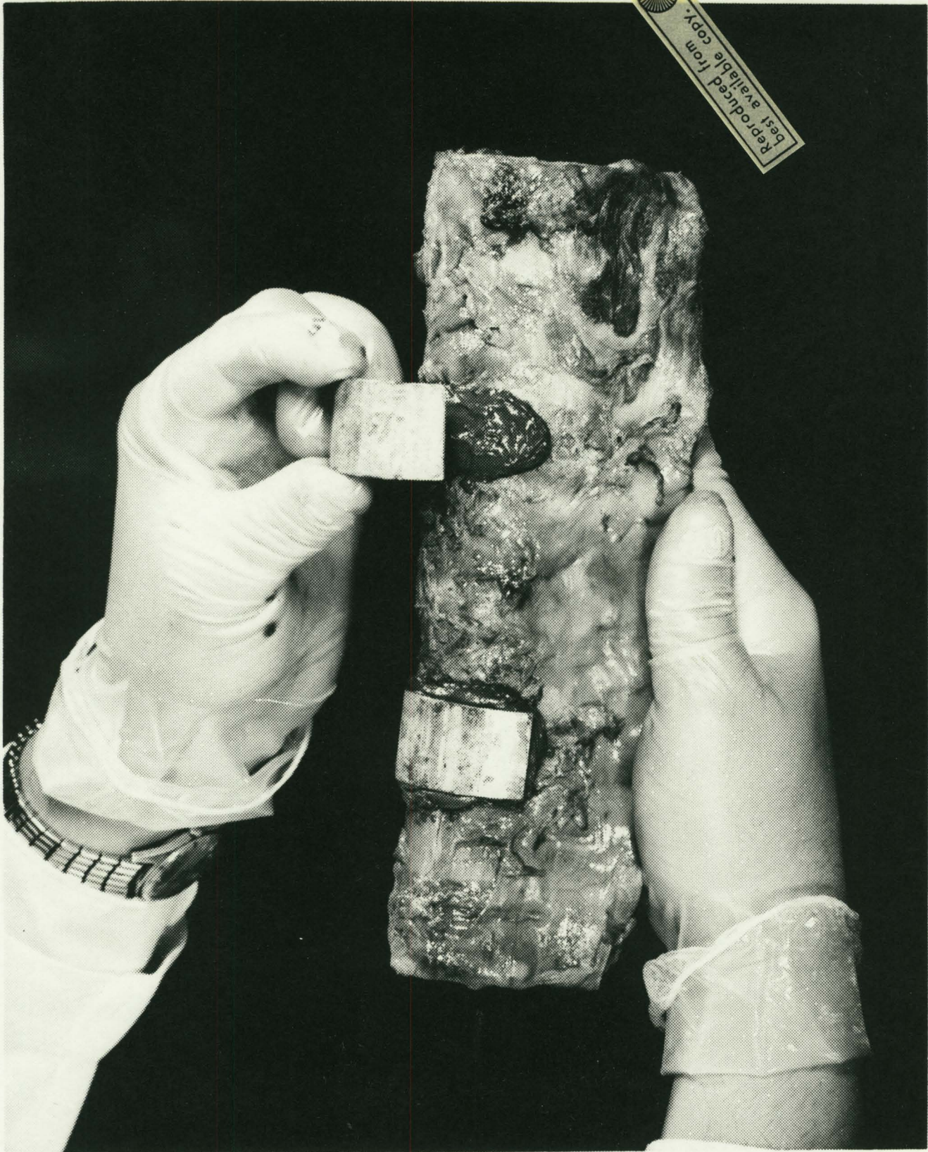
Fig. 1 Positioning of load distributing clamps on a segment of fresh, unembalmed, human vertebral column.
