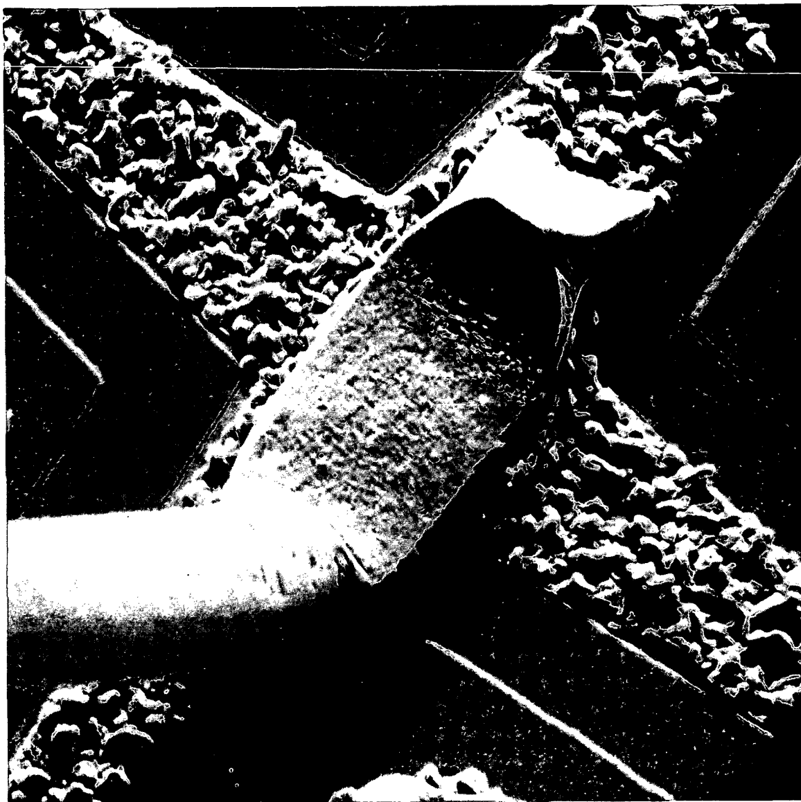
Frontispiece — Scanning electron microscope photomicrograph (magnification \sim 920\times ) of an aluminum-aluminum ultrasonic wire bond after 76,000 power cycles. The bond was made with large loop height to reduce the flexure fatigue of the aluminum wire during power cycling. The pronounced hillock growth on the aluminum metallization also results from the power cycling. (See section 4.2)
