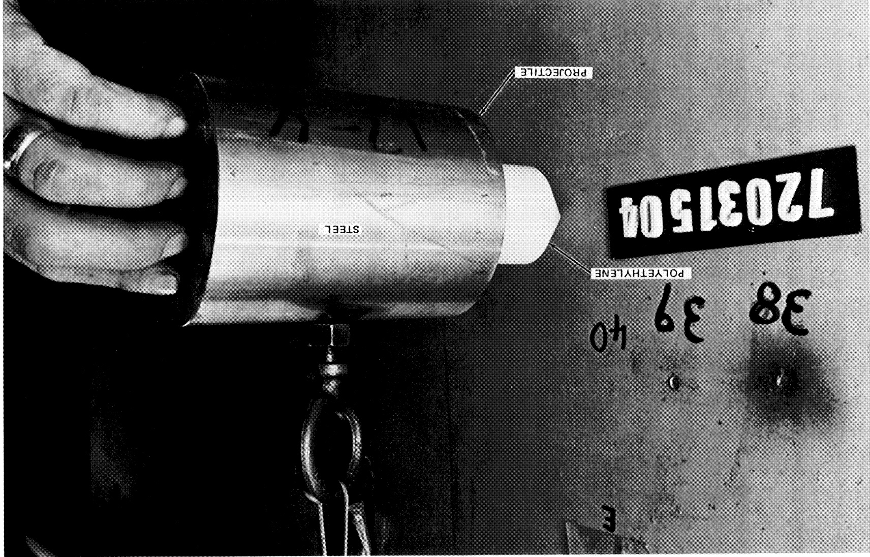
Figure 4-47. Projectile used for Ballistic Pendulum-Type Impacts on Large Target Sheet
