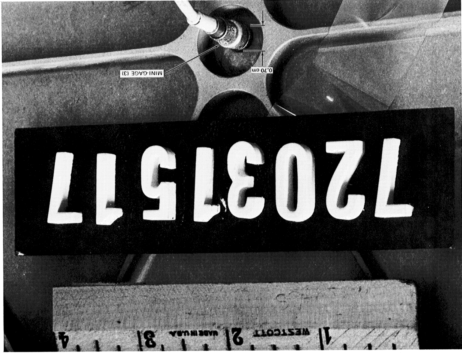
Figure 4-41. Miniature Impact Gage (3) Model A Installed on Isogrid Wall of 8-Foot-Diameter Delta Tank
