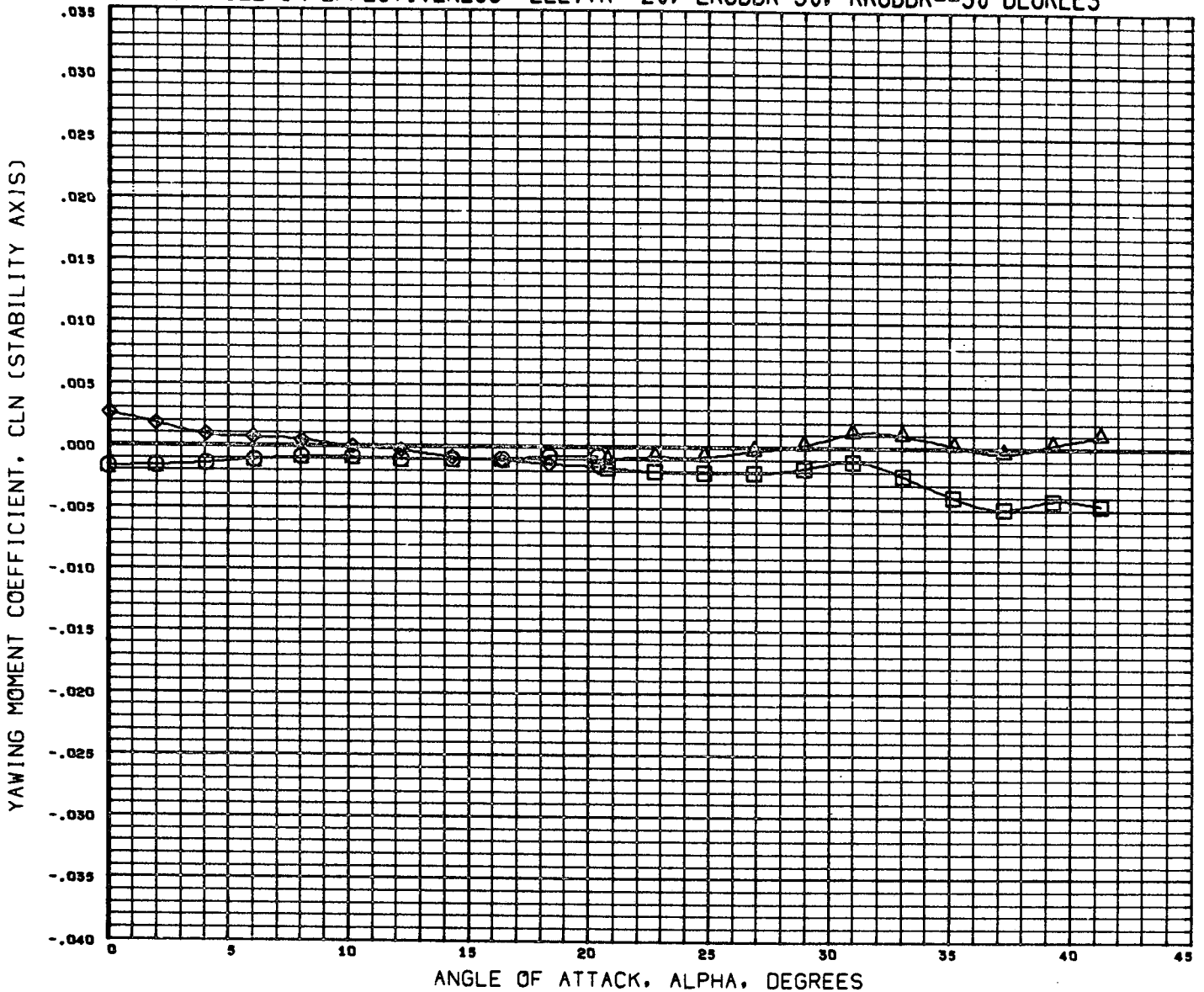
FIGURE 5, AILERON EFFECTIVENESS- ELEVTR=-20, LRUDDR=30, RRUDDR=-30 DEGREES
