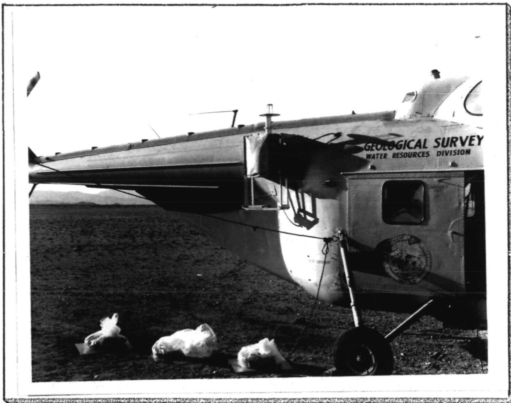
Figure 1. FLD mounted on H-19 helicopter during tests of response to fluorescent granules, Needles, Calif.
