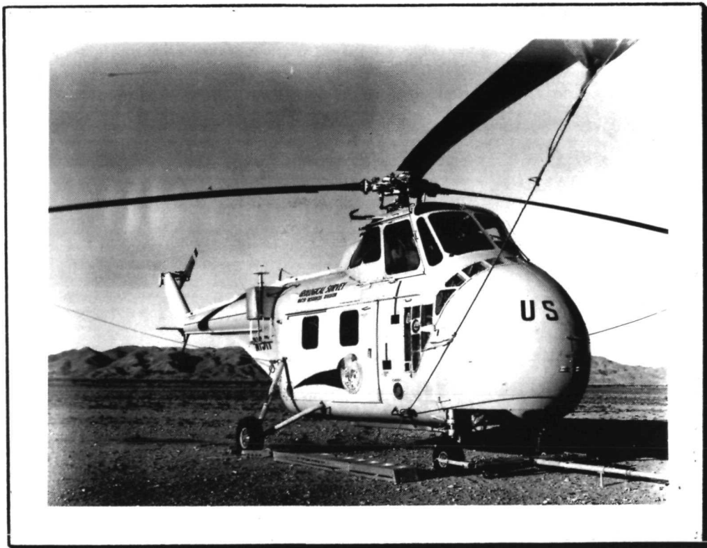
Figure 2. FLD mounted on H-19 helicopter for test over evaporite minerals in Death Valley (December, 1969, Needles, California)
