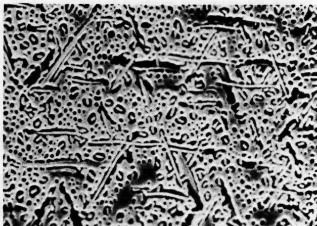
(h) ALLOY 17 - Cr NEEDLES ETCH: MIXED ACIDS
