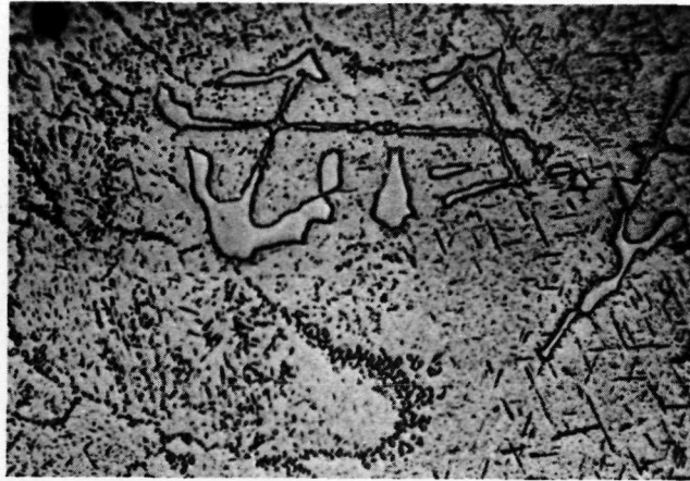
(k) ALLOY 6 - SIGMA AND W PHASES ETCH: KOH
