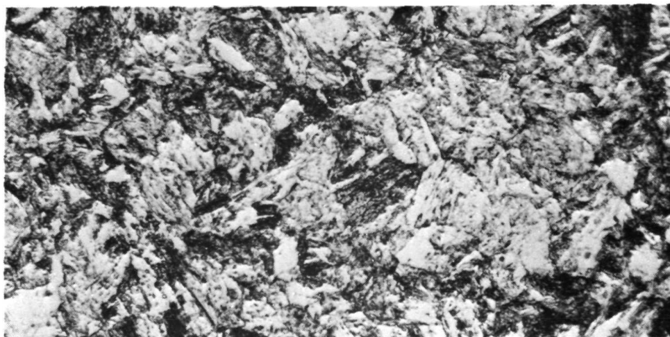
Fig. 8 - Microstructure of 1-inch plate of 10Ni-8Co-2Cr-1Mo steel (1000X, 2% Nital etch)
