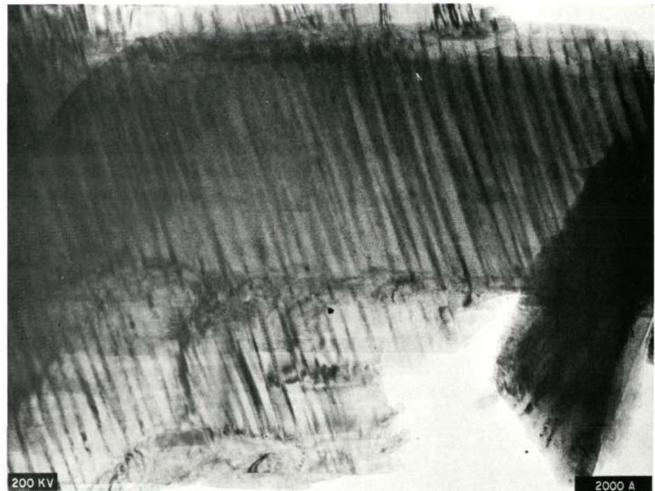
HIGH VOLTAGE ELECTRON MICROGRAPH OF MAGNESIUM RICH LUNAR PYROXENE 10044 SHOWING IRREGULAR STRIATIONS
