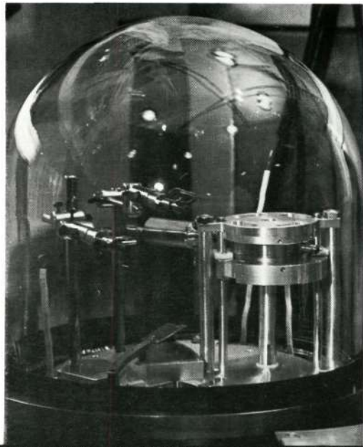
SPECIAL ULTRAHIGH VACUUM CHAMBER FOR CONTROLLED MANIPULATION AND EXAMINATION OF LUNAR SAMPLES.
