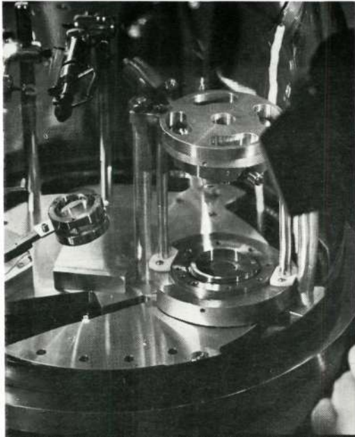
SPECIAL ULTRAHIGH VACUUM CHAMBER FOR CONTROLLED MANIPULATION AND EXAMINATION OF LUNAR SAMPLES.
