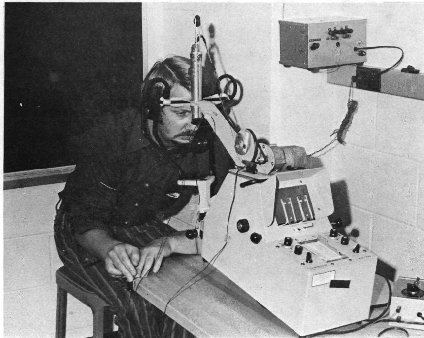
Fig. 13b. Modified Biometric Eye Trac Eye Movement Device with Subject in Place.
