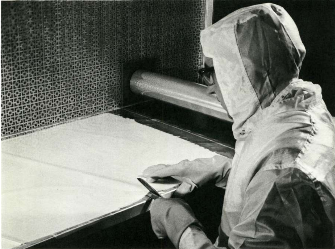
Figure 4. CUTTING TEFLON CLOTH ON A CLASS 100 HORIZONTAL-FLOW CLEAN BENCH.
