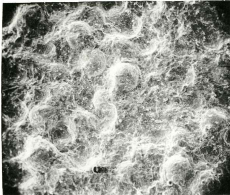
Figure 5.19 3-Hour Pressure/Temperature Shutdown Cycle. Type 8 Cermet (200x).
