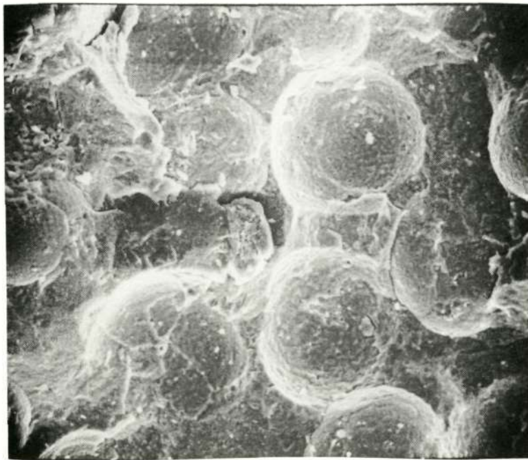
Figure 5.12 3-Hour Pressure/Temperature Shutdown Cycle. Type 7 Cermet (3000x).
