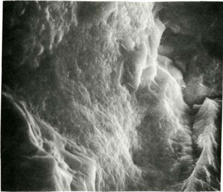
Figure 5.12 3-Hour Pressure/Temperature Shutdown Cycle. Type 7 Cermet (3000x).
