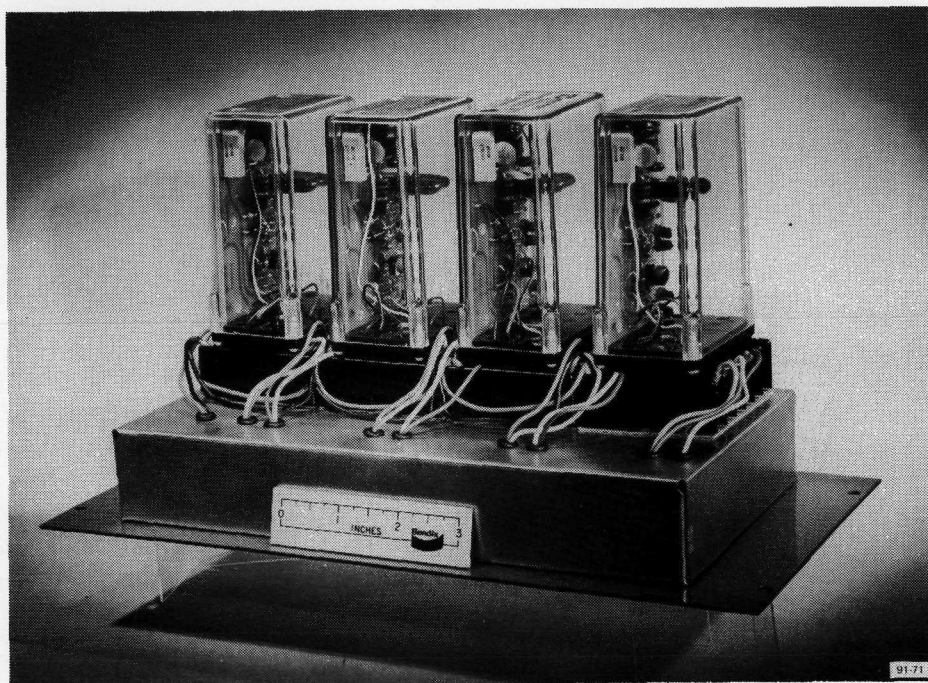
Figure 5-16 - Photograph of Commercial Sensor - Driver Circuit Modules
