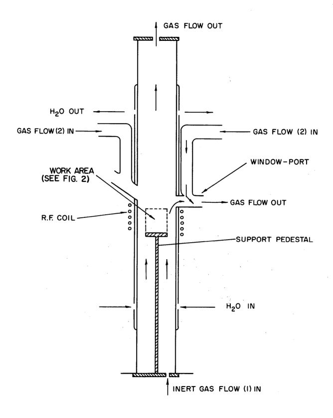
Fig. 10. Quartz furnace assembly incorporating two window ports
