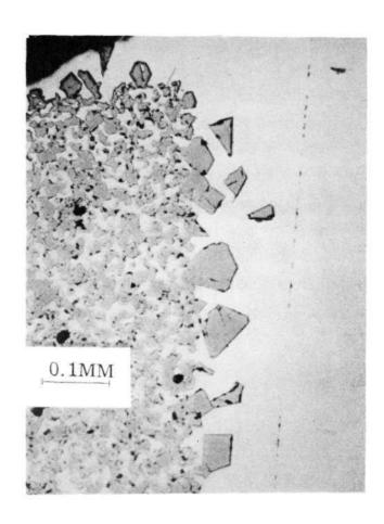
Fig. 2. Photomicrograph of SiC-Si interface along the capillary feeding channel of the EFG die (note morphology of SiC crystals at the SiC-Si interface)
