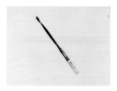
Fig. 8. EFG-grown silicon ribbon showing crystallographic flats developed on one side during growth at approximately  $20 \, \text{in./hr}$
