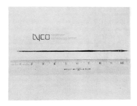
Fig. 5. Single crystal silicon ribbon grown from the melt by EFG (ribbon thickness is  $0.5\ \text{mm}$ )
