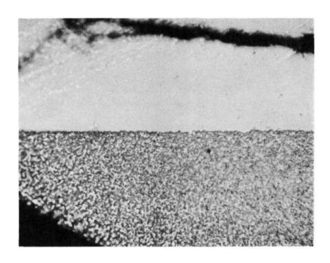
Fig. 4. Photomicrograph of interface between Si and SiC/10% SiO  $_2$  near the top of an orifice (140X)
