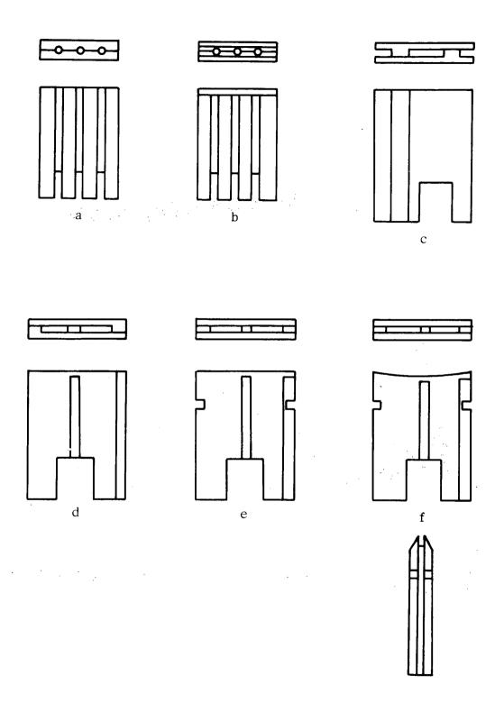
Fig. 3. Orifice configurations used in growing Si ribbons. Views are of the top surface and the inside of one side of the orifice. The side view of (f) is intended to show the knife edge bevel which was also used on some type (e) orifices. Typical overall dimensions for type c-f orifices are 0.7 in.  $\times$  0.4 in.  $\times$  0.065 in
