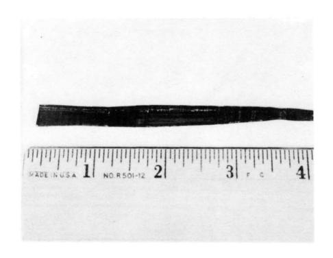
Fig. 7. Silicon ribbon showing a relatively smooth surface on one side of the long axis roughness caused by orifice disintegration on the other
