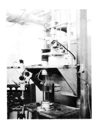
Fig. 11. Crystal growth apparatus
