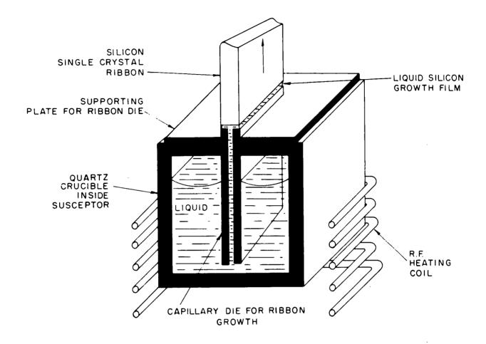
Fig. 1. Schematic drawing showing crucible and die arrangement for edge-defined, film-fed growth (EFG) of silicon ribbon
