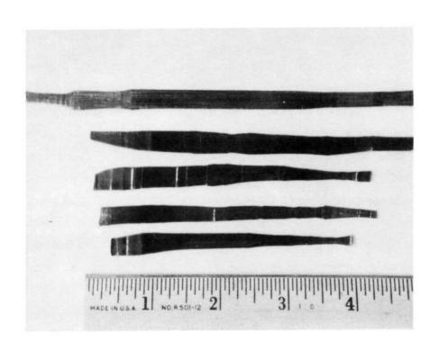
Fig. 6. EFG-grown silicon ribbons of the order of 8 to 9 mm in width
