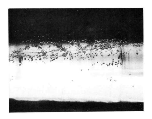
Fig. 9. Dislocation etch pits in EFG-grown silicon ribbon showing variable distribution across the width of a single riboon (Dash etch,  $35\,\mathrm{X}$ )
