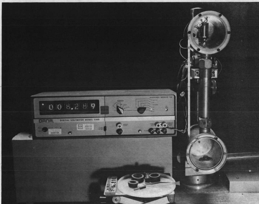
Figure 13. System Being Developed for Drying and Weighing Arc Chamber Parts in a Continuous Vacuum
