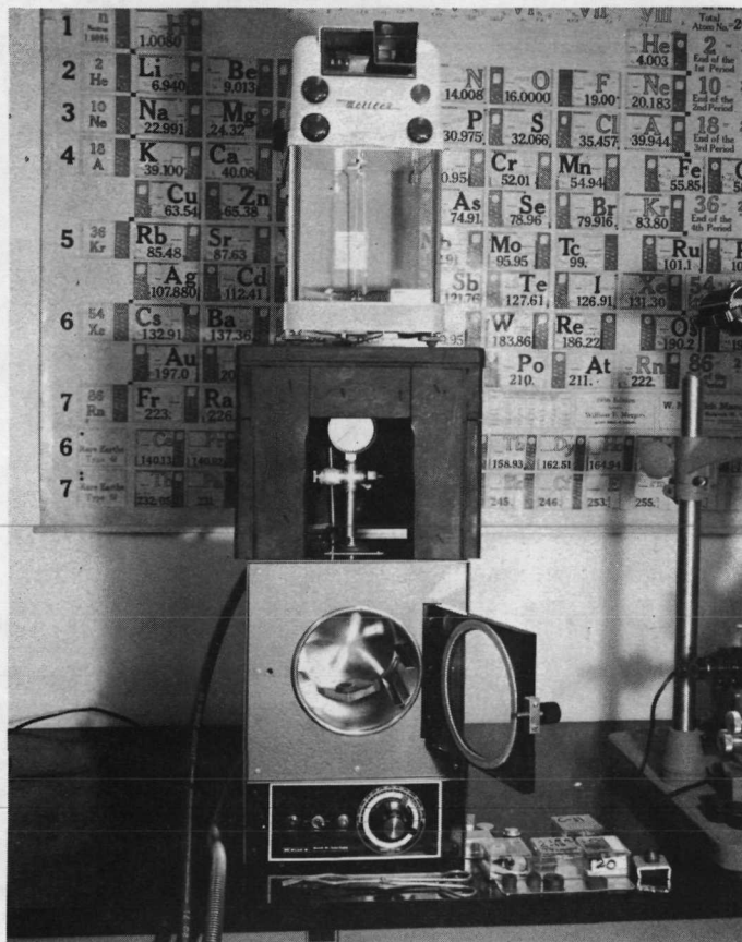
Figure 12. Setup of Vacuum Oven and Balance Used for Drying and Weighing Arc Chamber Parts
