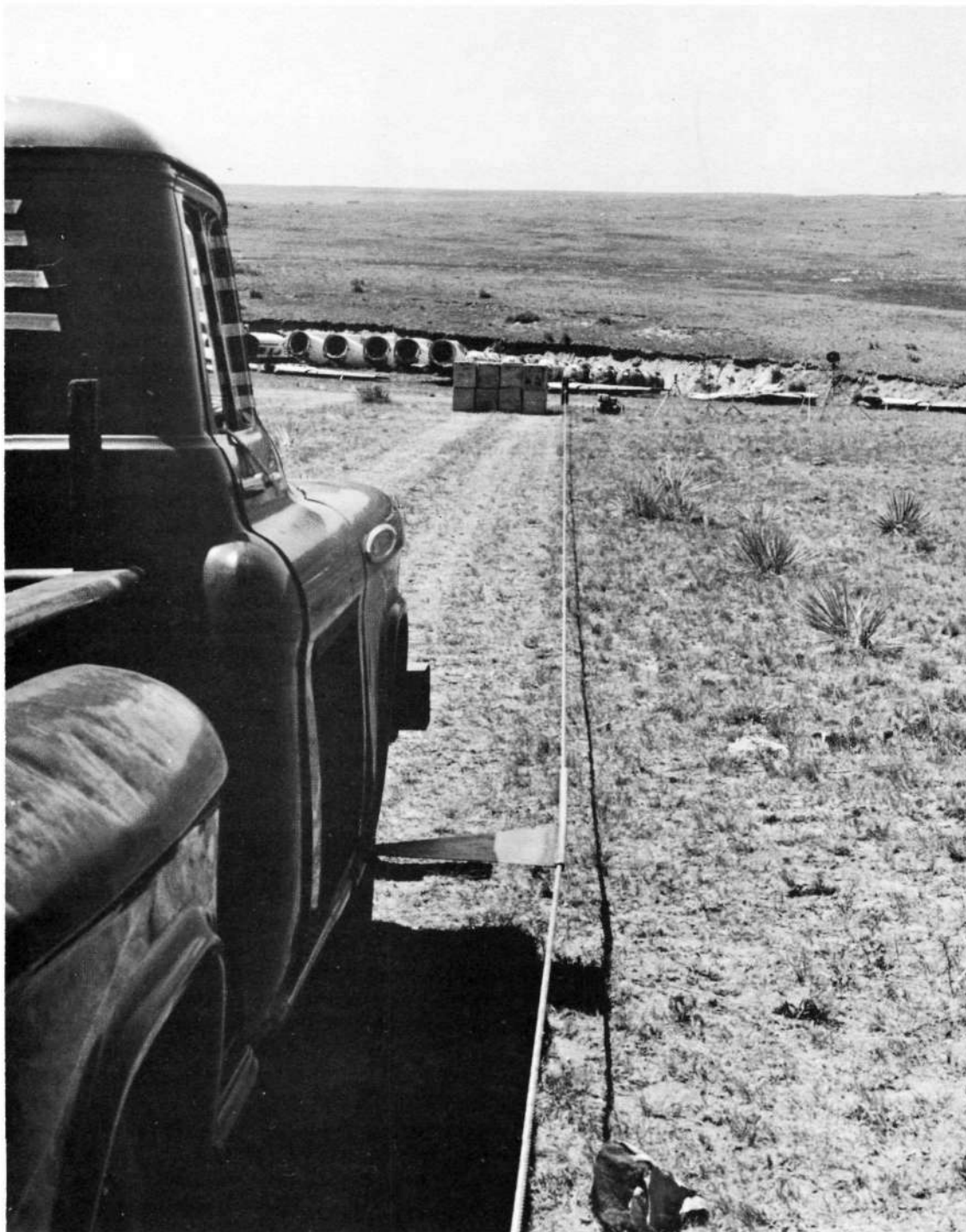
Figure 6.7. Test Track, Barrier, and Vehicle Guidance Cable.
