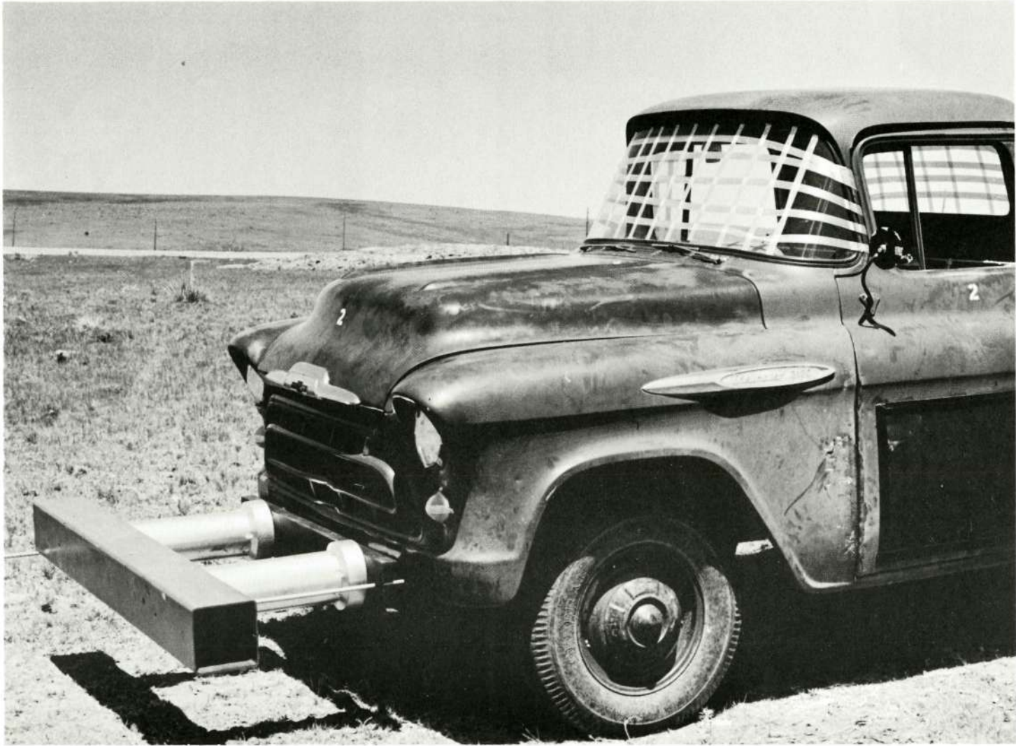
Figure 6.6. Bumper Mounted on Test Vehicle
