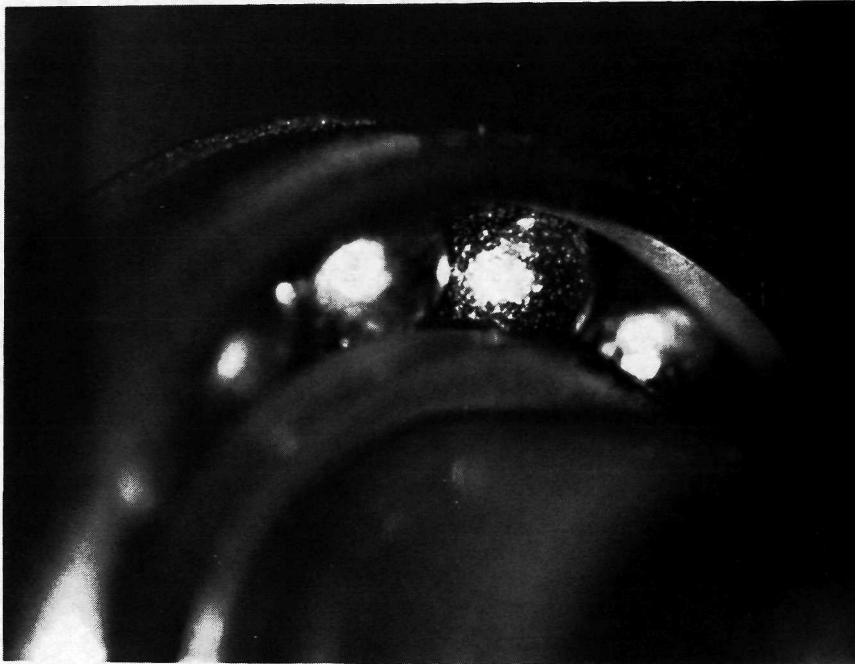
Figure 5. - Spalled ball bearing from type E-F meter; ball diameter, 0.8 millimeter.
