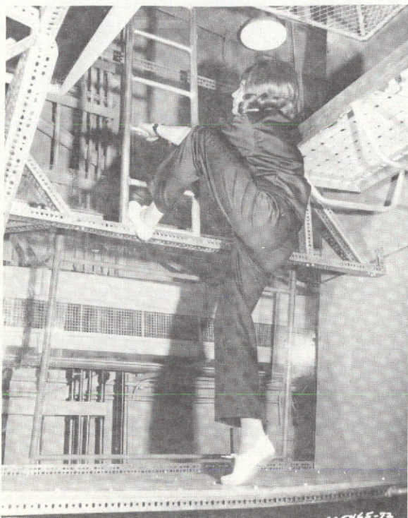
Figure IV-22 Female Test Subject Climbing from exit Hatch Deck to Upper Crew Compartment Area
