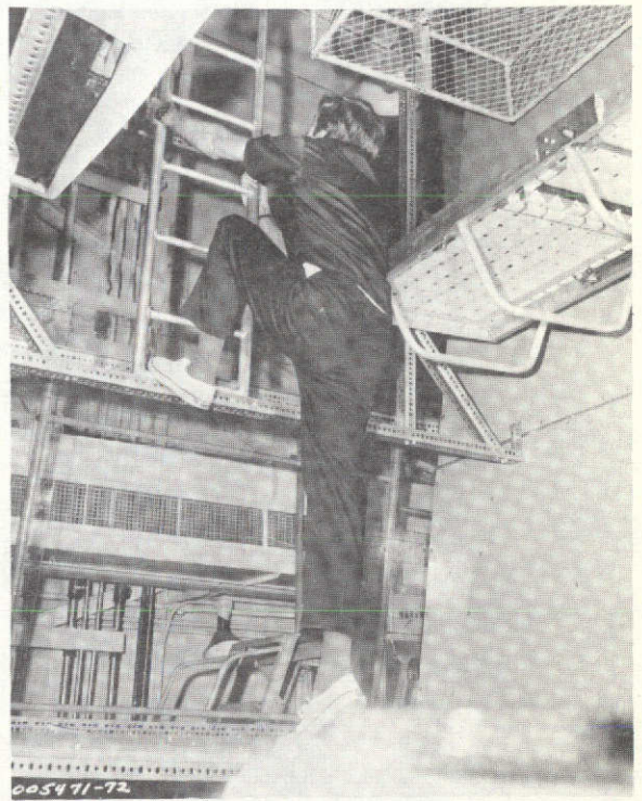
Figure IV-23 Male Test Subject Climbing from Exit Hatch Deck to Upper Crew Compartment Area
