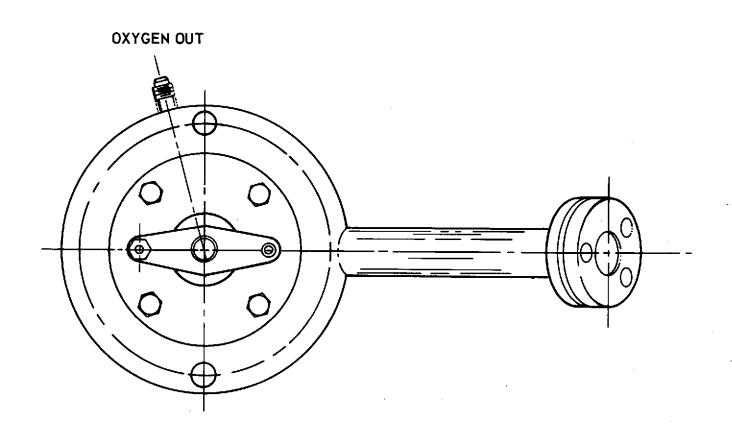
FIGURE 2. GOX IMPACT TESTER, TOP VIEW
