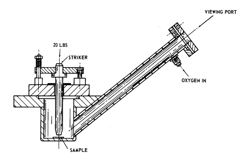
FIGURE 1. GOX IMPACT TESTER, SIDE VIEW
