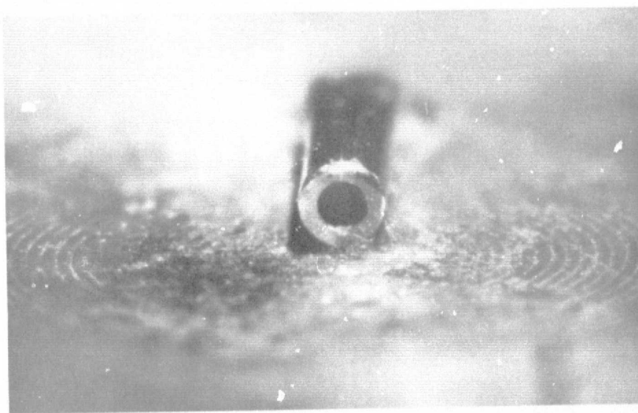
Photomicrograph (36.3 X) of the tip of the 0.018" dia Preston probe
