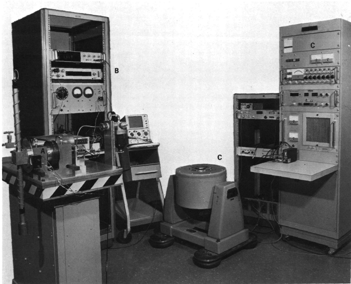
Figure 8. Apparatus used in the calibration of pressure transducers for pogo measurements. The windmill source is shown at (A) with supporting electronics in rack (B). The vibration-exciter system which forms part of the oscillating source is at (C).
