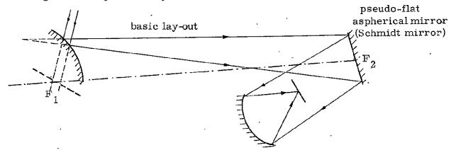
The object pupil of the instrument is the virtual image, in the hyperbolic mirror, of the real pupil of the Schmidt camera, symbolised by a diaphragm on the drawing. Thus, for each point of the field, the hyperbolic mirror functions over a small part of its surface.
