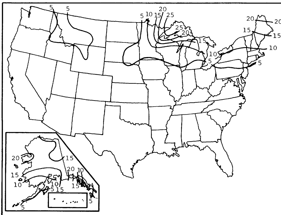
Figure 6.16 Snow load in lb ft -2 on the ground, 0.50 quantile, 2-year mean recurrence interval [6.9].
