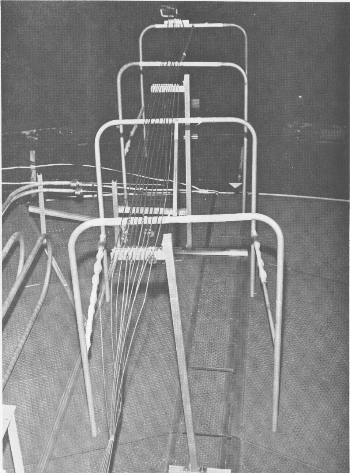
Figure 10. Gas line arrangement inside Chamber A.
