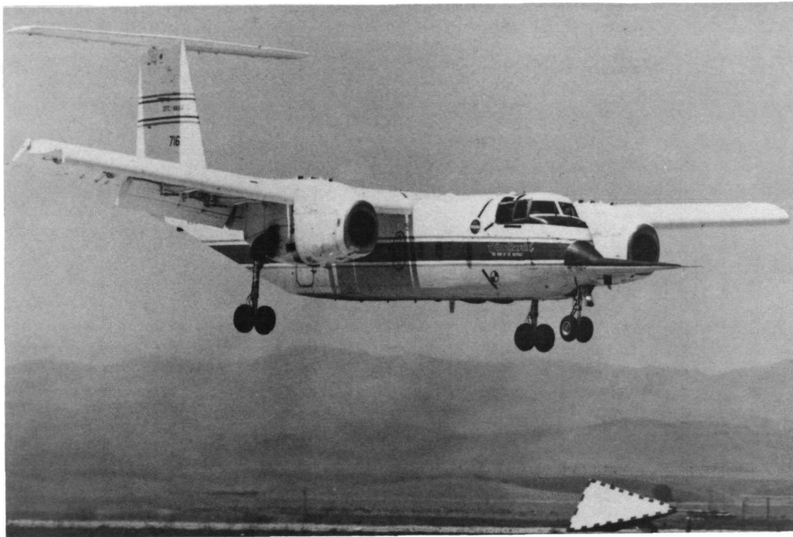
Figure 1.- Augmentor wing jet STOL research aircraft.
