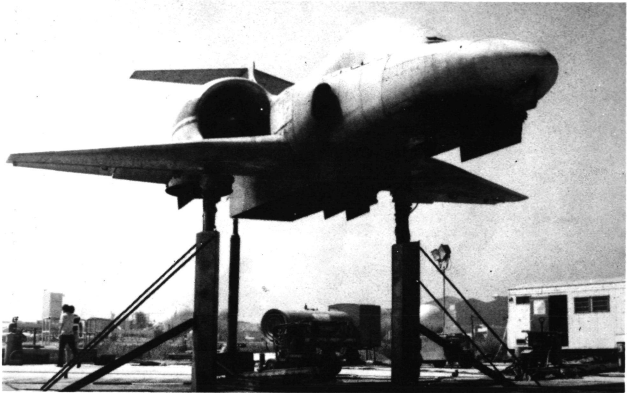
FIGURE 2-11 LID INSTALLATION ON LSPM
