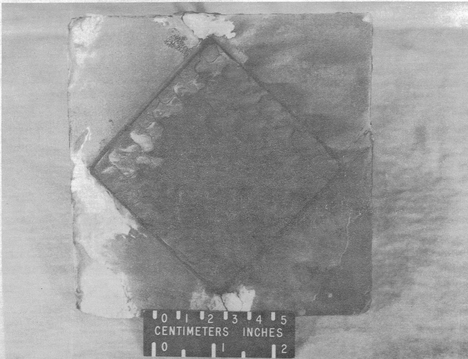
Figure 9.- Panel no. 5, ESA-3560 after 400s entry test at 20 Btu/ft 2 s.
